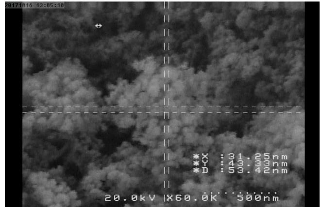
Fig. 1. SEM image of silica nanoparticles.
