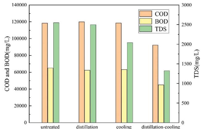
Fig. 6. Comparison histogram of TDS, COD<sub>Cr</sub> and BOD<sub>5</sub>.
