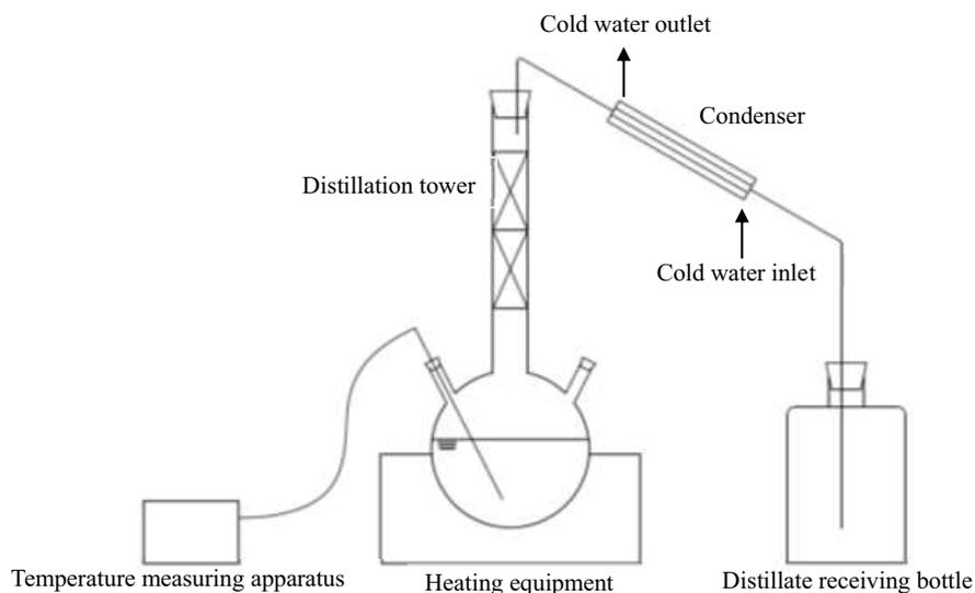
Fig. 1. Distillation experiment apparatus.
