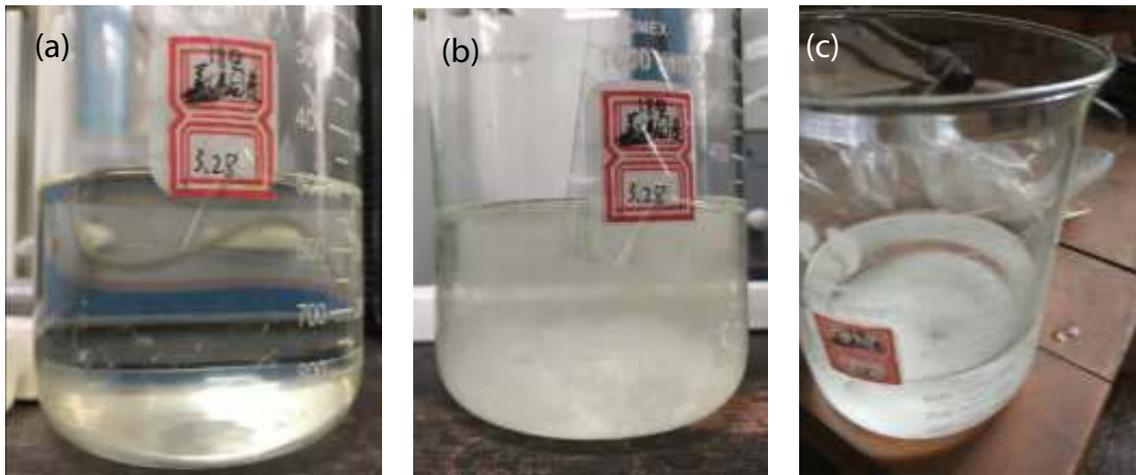
Fig. 4. (a) Wastewater by distillation, (b) Wastewater by distillation-cooling and (c) Wastewater treatment by distillation-cooling after 12 h.
