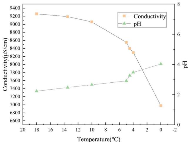
Fig. 5. Effect of temperature on conductivity and pH by distillation-cooling.
