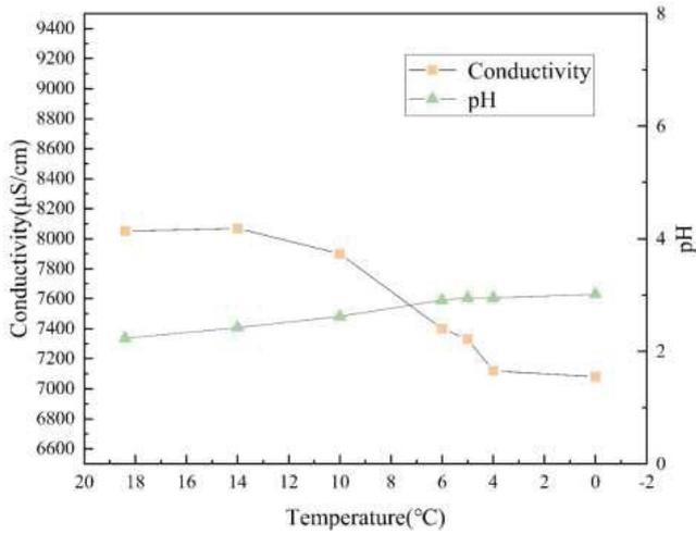
Fig. 2. Effect of temperature on conductivity and pH by cooling.
