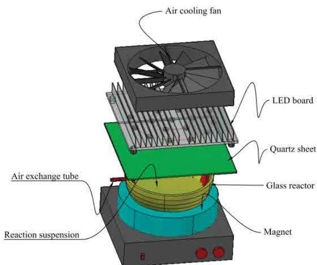
Fig. 2. 3D picture of the batch reactor under study.
