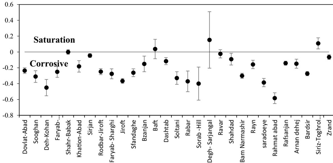
Fig. 2. Variations of the average and confidence interval ( $p < 0.05$ ) of the Langelier index compared with the stable condition in sampling locations.
