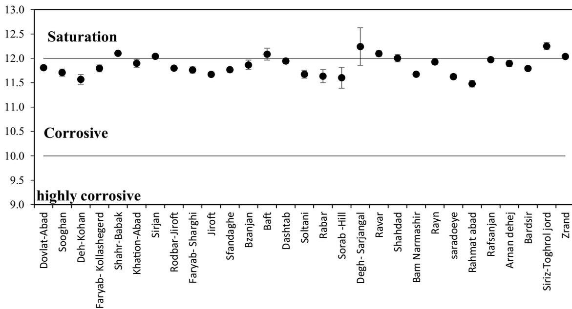
Fig. 5. Variations of the average and confidence interval ( $p < 0.05$ ) of the Aggression index compared with the stable condition in sampling locations.
