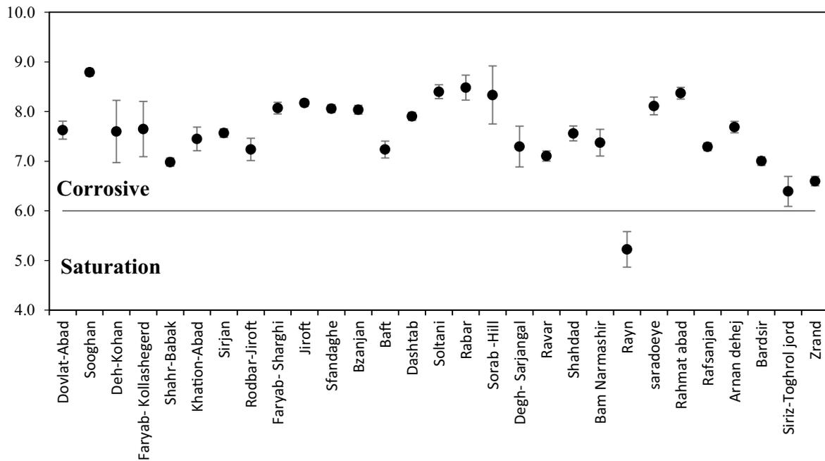
Fig. 4. Variations of the average and confidence interval ( $p < 0.05$ ) of the Puckorius index compared with the stable condition in sampling locations.
