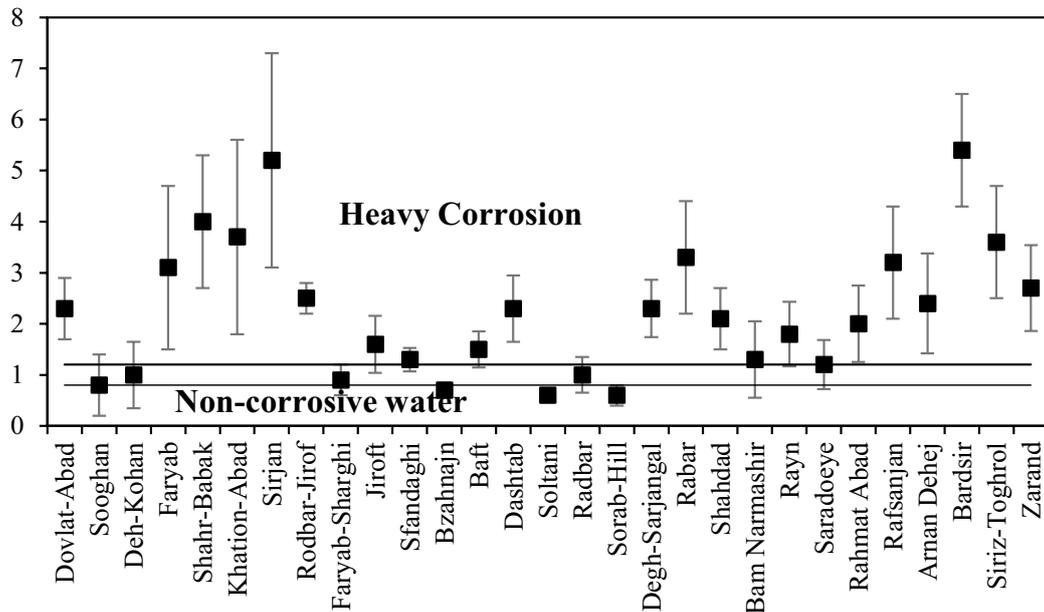
Fig. 6. Variations of the average and confidence interval ( $p < 0.05$ ) of the Larson–Skold index compared with the stable condition in sampling locations.
