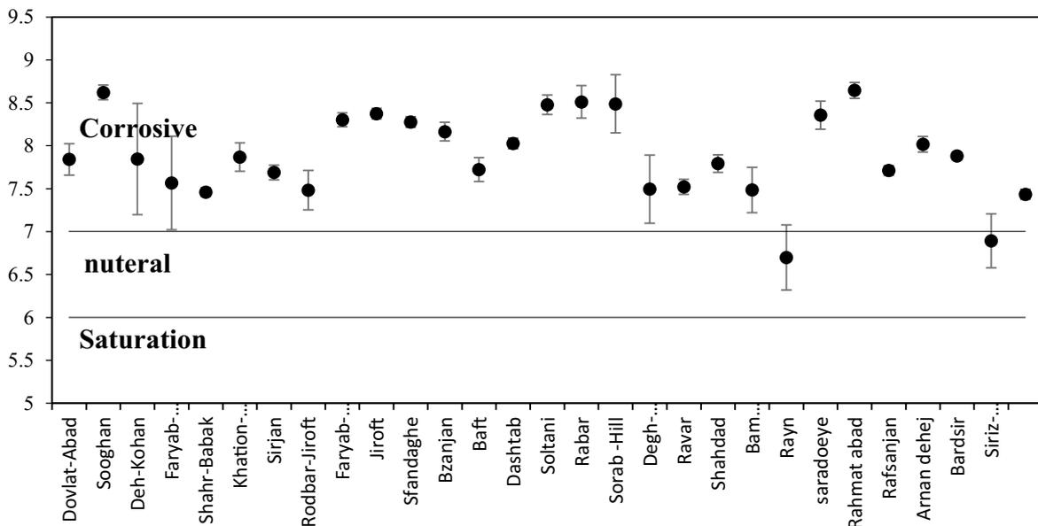
Fig. 3. Variations of the average and confidence interval ( $p < 0.05$ ) of Ryznar index compared with the stable condition in sampling locations.
