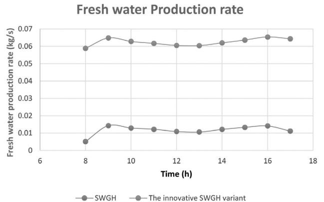
Fig. 9. Fresh water amounts produced by the basic SWGH and by the innovative one.
