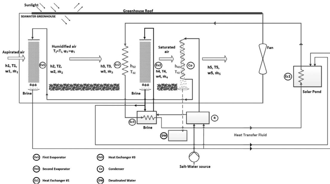
Fig. 2. Diagram of the innovative system – day operating mode.
