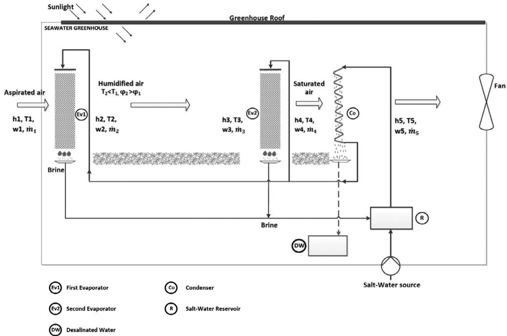
Fig. 1. Diagram of a basic seawater greenhouse.
