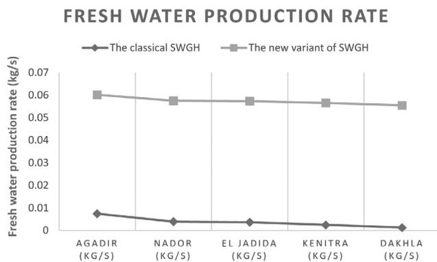
Fig. 10. Simulations results – estimated mean values of fresh water production rate for the basic SWGH and for the new one in different Moroccan locations.
