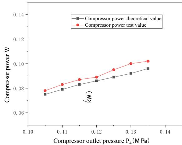
Fig. 7. Compressor power as a function of discharge pressure.
