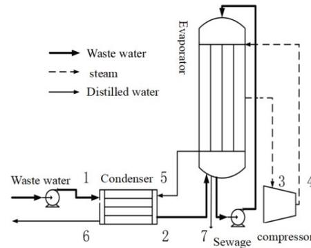
Fig. 1. MVR method to treat the water co-produced with oil design model.
