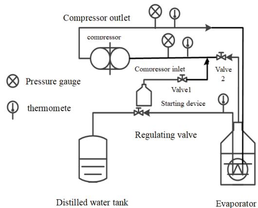
Fig. 3. Experimental system diagram.
