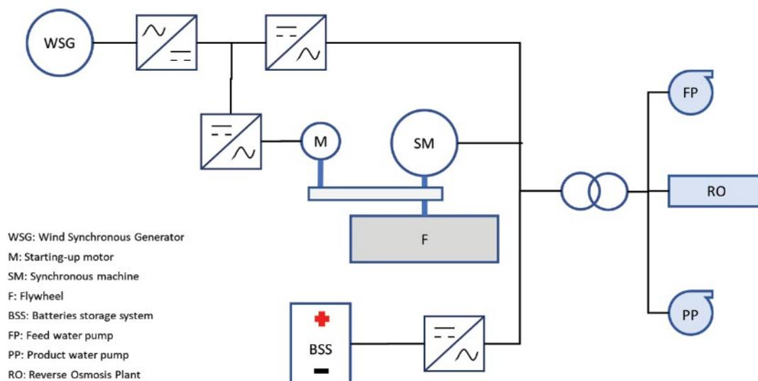
Fig. 1. Basic electric diagram of the generation system and loads.
