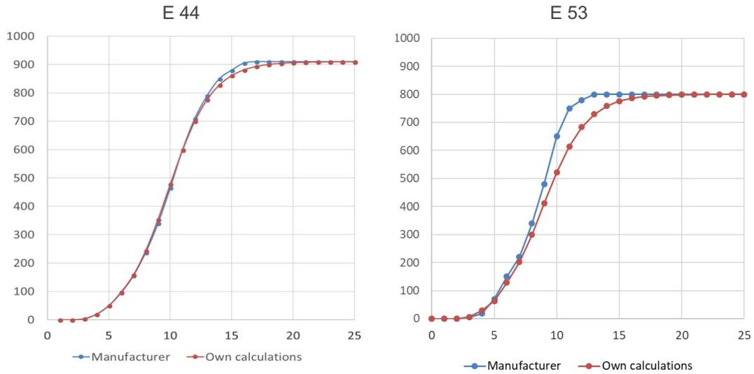
Fig. A.1. Chart and data of output power curves (real form the manufacturer, and estimated), in kW vs. wind speed, in m/s.
