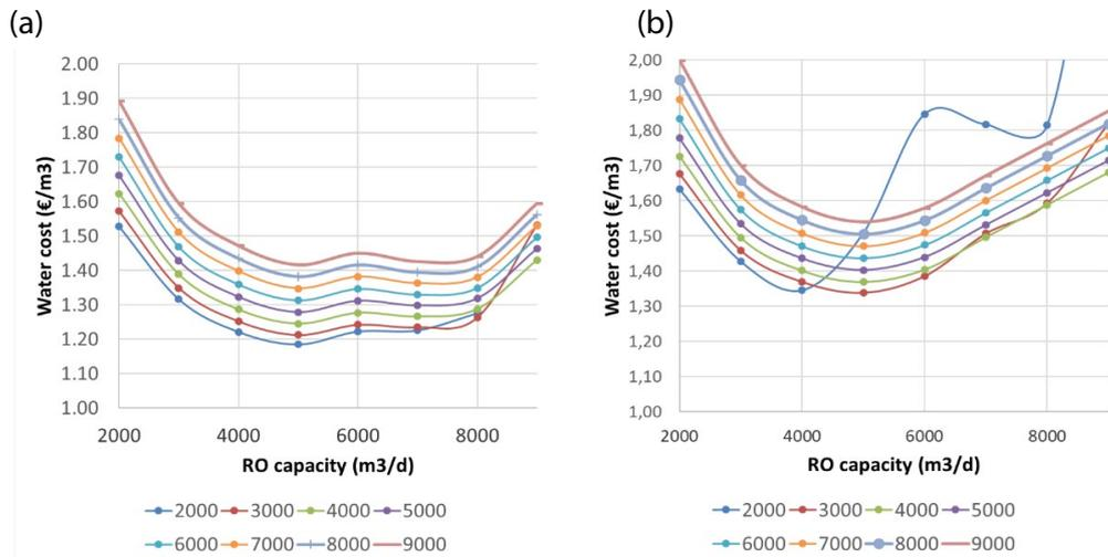
Fig. 10. Water cost vs. RO capacity for different energy storage sizes (in Ah): (a) Case 1, (b) Case 2.
