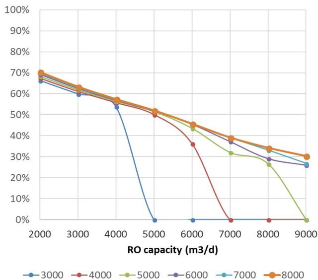
Fig. 11. Reference case: percentage of operation time vs. the nominal capacity of the RO plant ( $\text{m}^3/\text{d}$ ) for different capacities of batteries (Ah).
