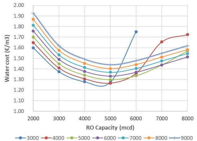
Fig. 9. Chart of water cost against RO capacities as a function of capacity of batteries (Ah) (Case 0).
