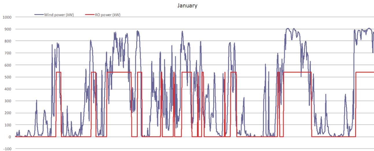
Fig. 6. Power evolution in January for the Case 0 – Reference Case- (operation under a minimum time of 8 h)
