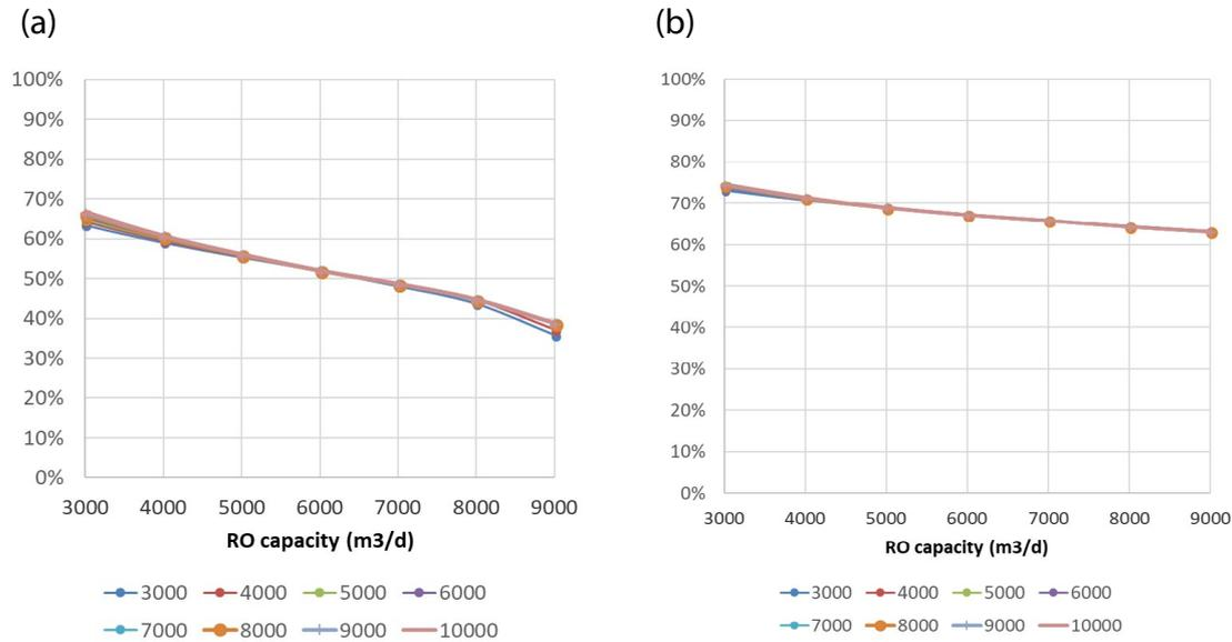
Fig. 12. Annual operation time vs. RO capacity for different energy storage sizes (Ah) ((a) Case 1, (b) Case 2).
