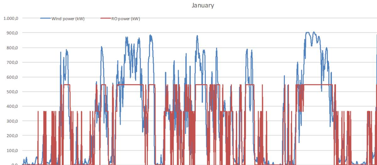
Fig. 7. Power evolution in January for the case 1 – variable operation of high-pressure pump- (option of discontinuous operation)
