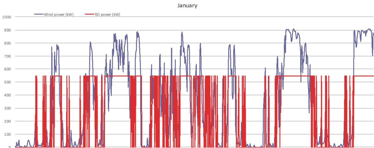
Fig. 5. Power evolution in January for the case 0 – reference case- (option of discontinuous operation).
