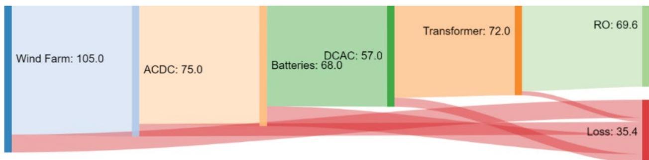
Fig. 3. Example of the energy flows through the main elements of the system.
