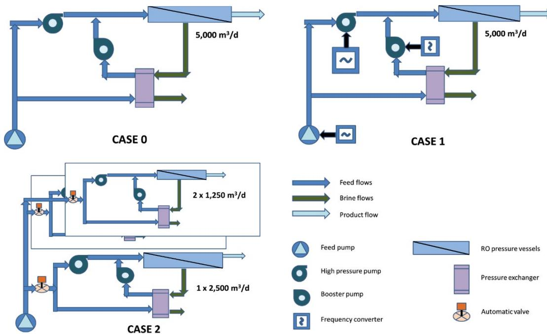
Fig. 2. Basic hydraulic diagrams of the RO configurations or cases.
