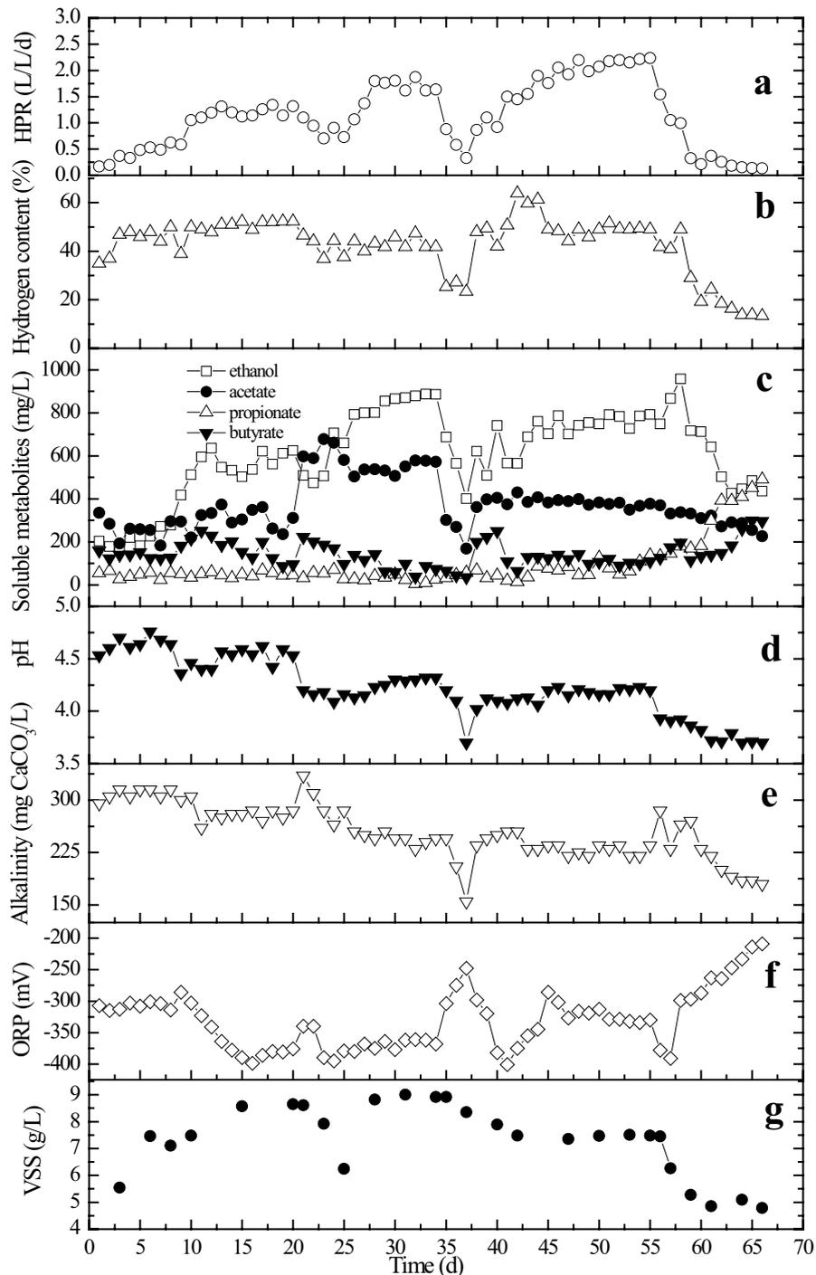
Fig. 2. Performance of hydrogen production in the ICSTR.
