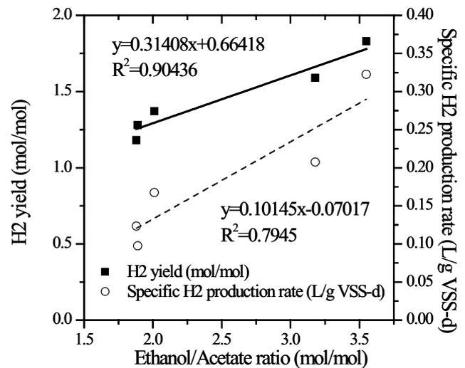
Fig. 4. Hydrogen yield and specific hydrogen production rate at different ethanol/acetate ratios.
