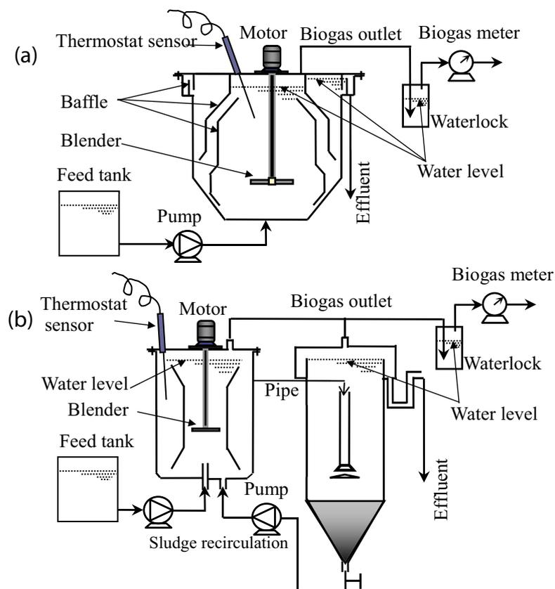
Fig. 1. Schematic diagram of the continuous reactor systems for hydrogen production (a) CSTR with inner three-phase separator and (b) anaerobic contact reactor.
