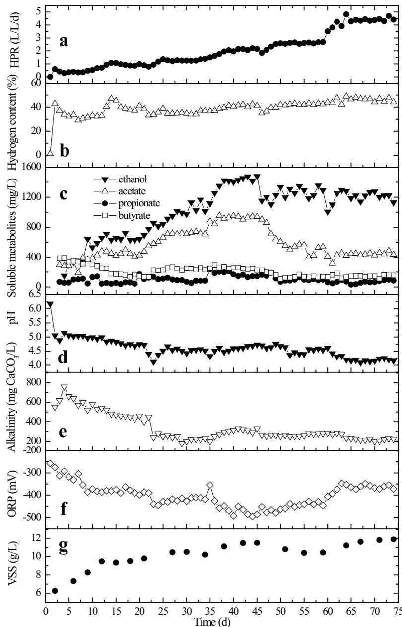
Fig. 3. Performance of hydrogen production in the ACR.
