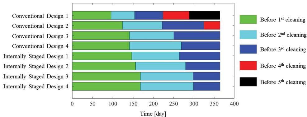
Fig. 4. Cleaning schedules depending on the membrane configuration. Different colors indicate the operation periods of the SWRO process before membrane cleanings.
