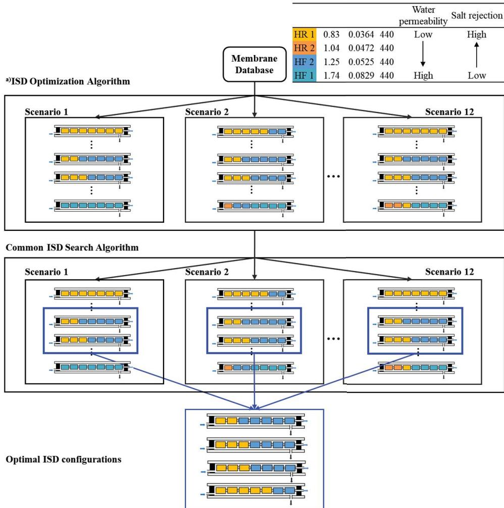
Fig. 2. Graphical summary of the internally staged design (ISD) optimization algorithm depending on the seasonal variations of seawater quality; HR: high rejection membrane; HF: high flux membrane; <sup>a)</sup>ISD optimization algorithm using the pattern search algorithm developed in our previous study.
