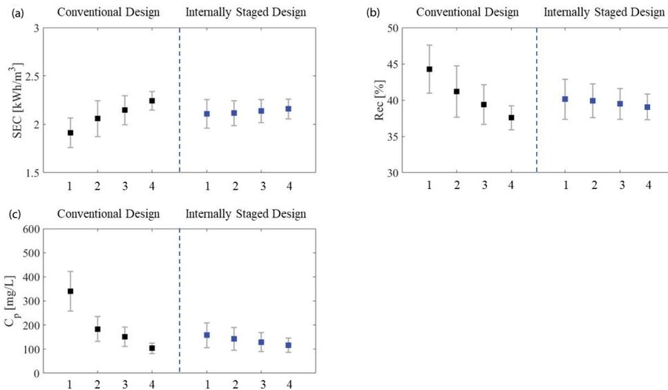
Fig. 3. Seawater reverse osmosis (SWRO) model simulation results for each element configuration: (a) specific energy consumption (kWh/m<sup>3</sup>), (b) recovery ratio (%), and (c) permeate TDS concentration (mg/L). The squares indicate the mean of each parameter. The error bars represent one standard deviation above and below the mean values.
