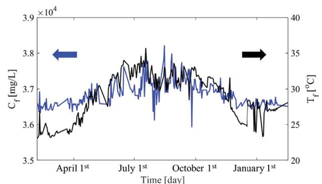
Fig. 1. Graphical illustration of seawater temperature and total dissolved solids (TDS) concentration in the intake of the Fujairah desalination plant during the 12-month observation period.
