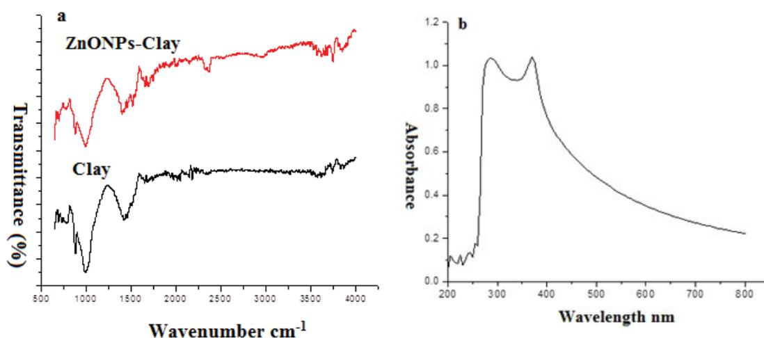
Fig. 1. FTIR (a) and UV (b) spectra of silty clay and ZnONPs-clay.
