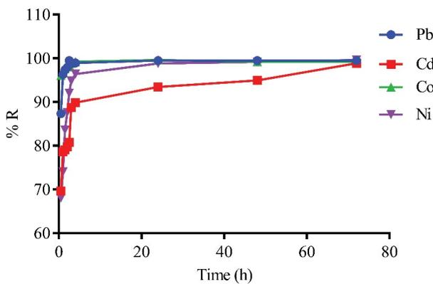
Fig. 4. % Removal of Pb(II), Co(II), Cd(II) and Ni(II) ions with time (h).
