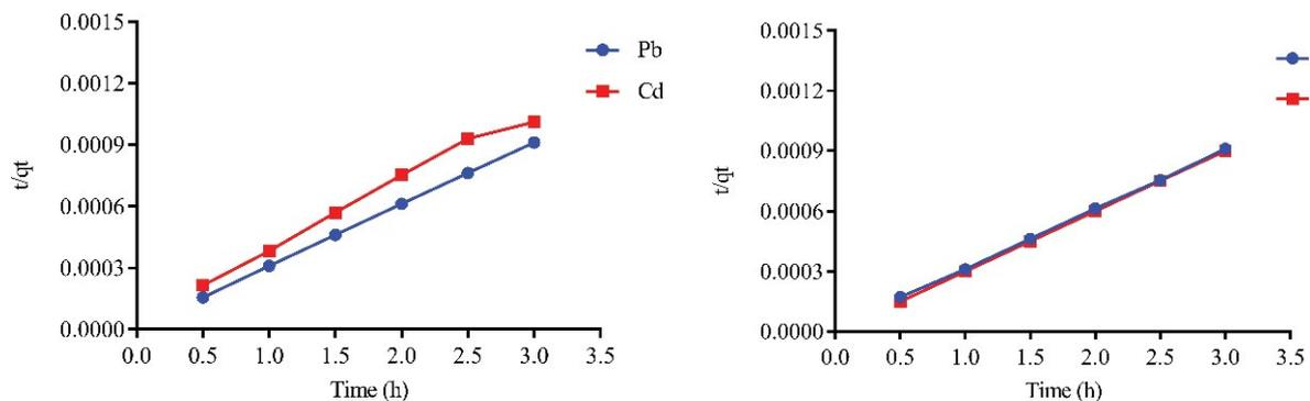
Fig. 5. Kinetic studies of the removal of Pb(II), Co(II), Cd(II), and Ni(II) ions with time (h).
