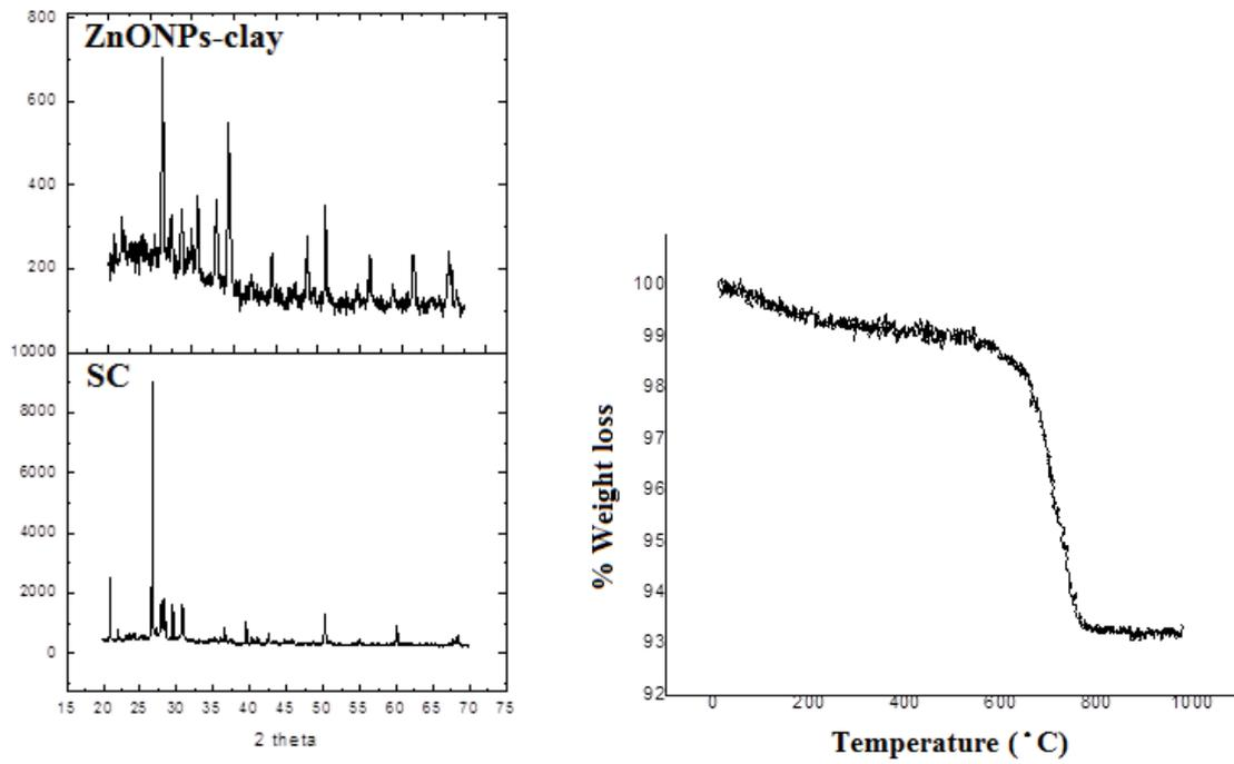
Fig. 2. XRD spectra of SC and ZnONPs-clay and TGA analysis of ZnO-clay tablet.
