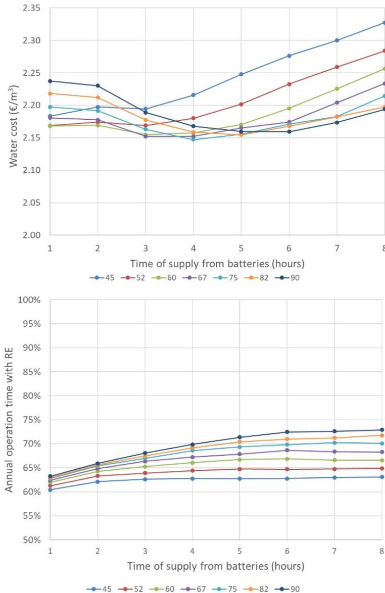
Fig. 10. Variation of water cost (top chart) and operation under RE supply (bottom chart) for different values of battery capacity (in hours of supply) and PV power (in kW).
