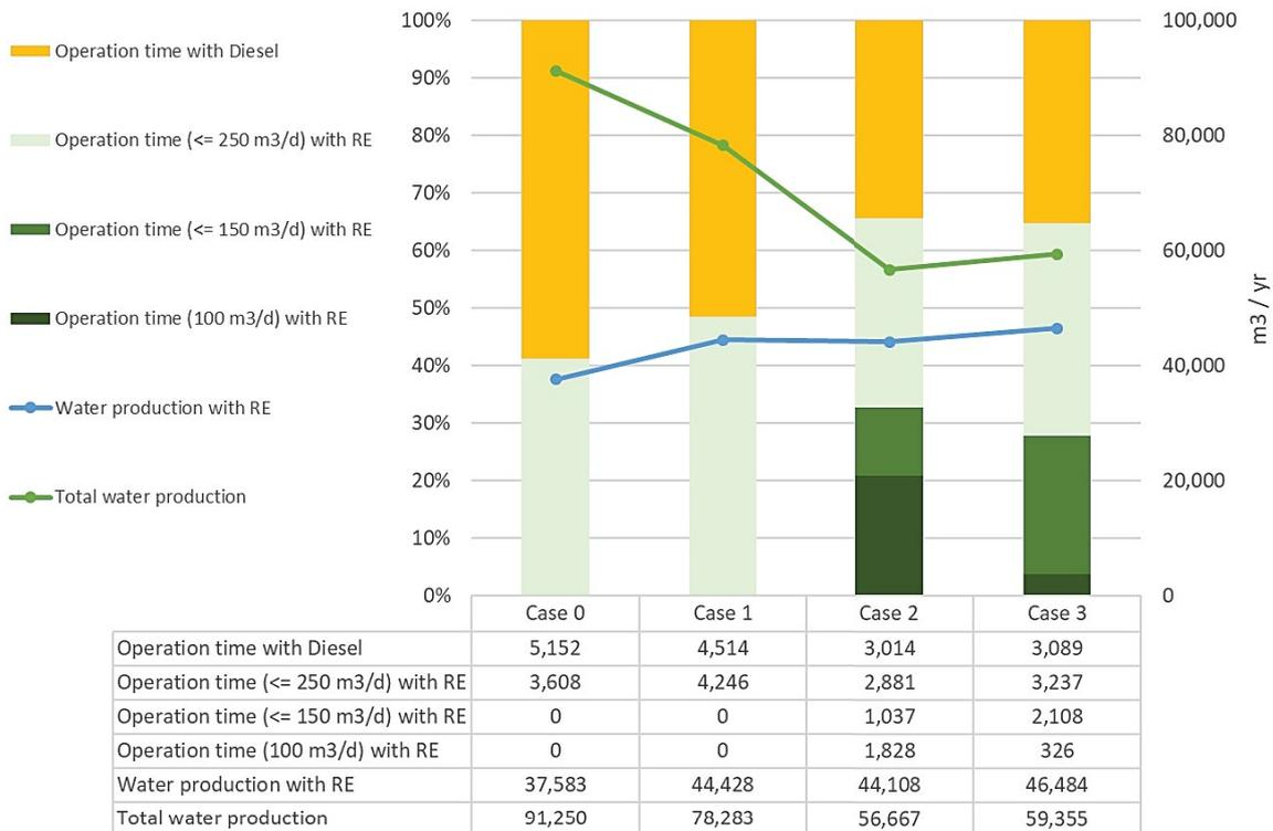
Fig. 9. Operation time (in hours per year) and water production (m³/a) for each case and type of energy supply.
