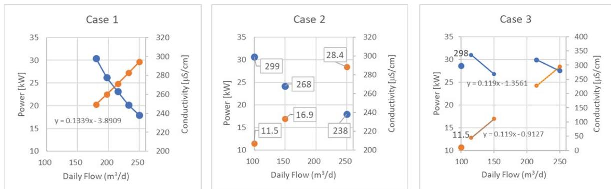
Fig. 6. Charts illustrating the operation points of the SWRO plant for each case (Power: orange points; Conductivity: blue points).
