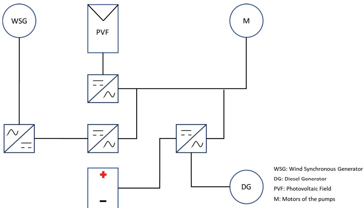
Fig. 2. Electric diagram of the system (simplified version).
