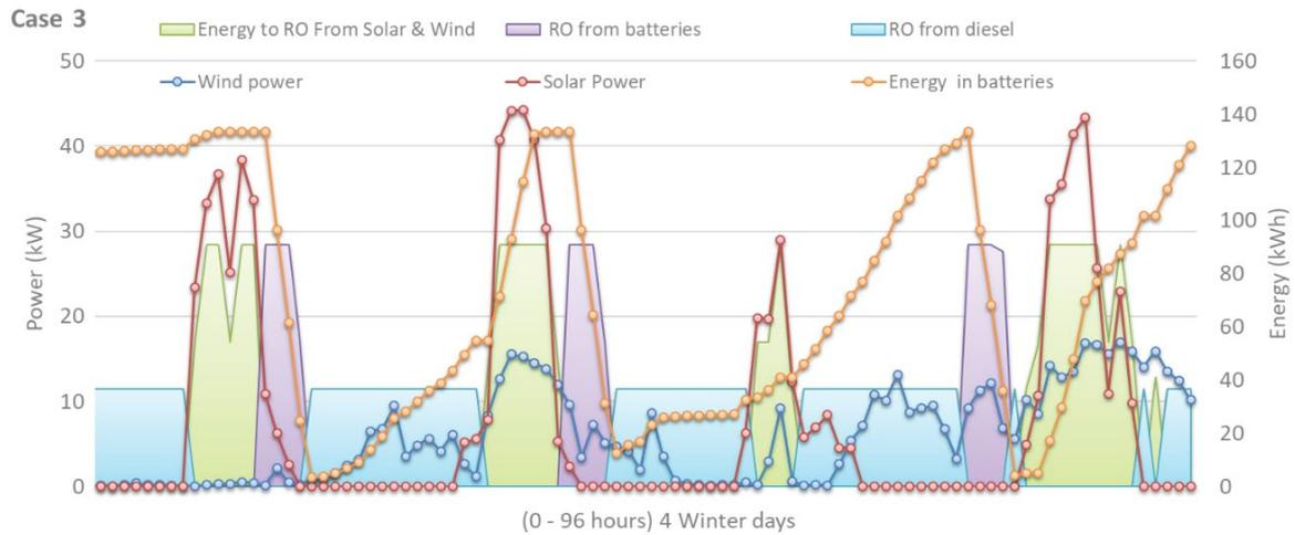
Fig. 8. Chart with the generated power (wind, solar PV), connection of RO, and energy in batteries (4 winter days) for case 3 (variable modular operation).
