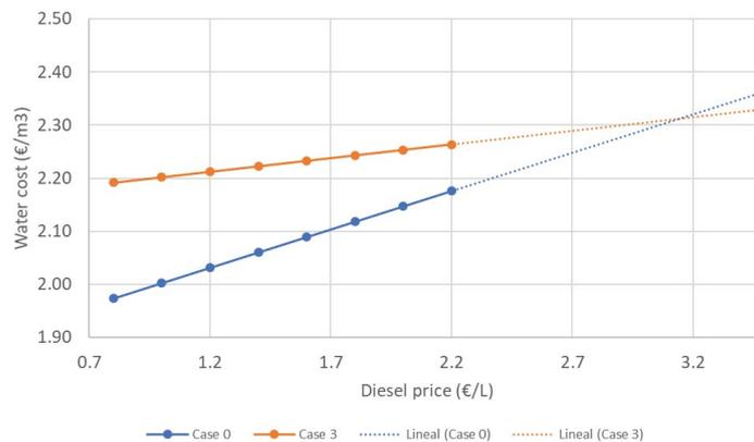
Fig. 12. Possible evolution of water cost as function of diesel cost.
