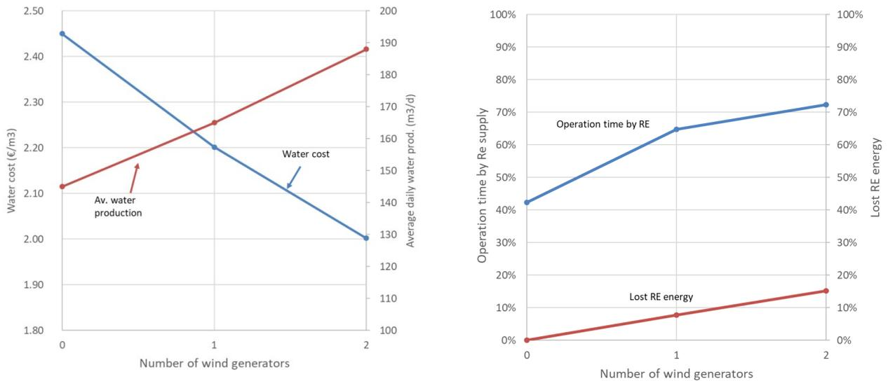
Fig. 11. Influence of a number of wind generators in the water cost, average water production, operation time by RE supply and lost RE energy.
