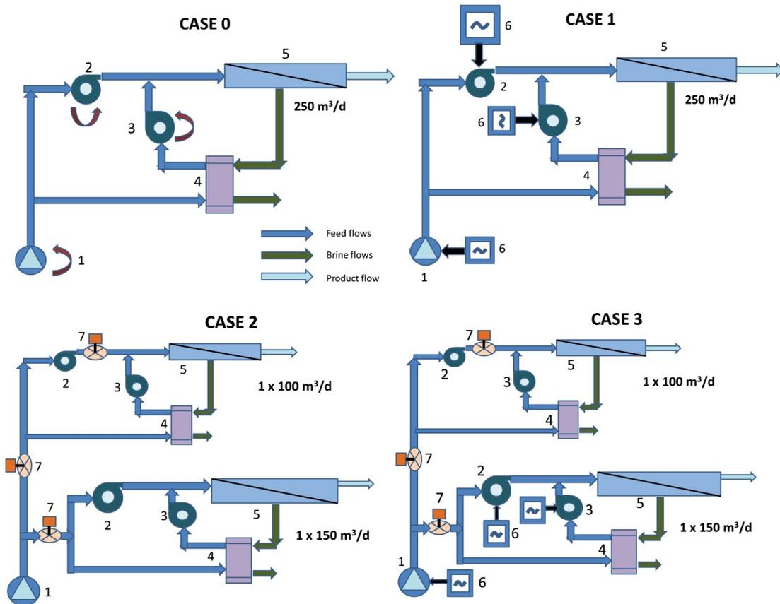
Fig. 3. Basic hydraulic diagrams. Case 0 (Reference case): RO unit of 250 m<sup>3</sup>/d operating at the nominal point. Case 1: RO unit of 250 m<sup>3</sup>/d with variable operation. Case 2. Modular RO unit (100 + 150 m<sup>3</sup>/d) at the nominal point. Case 3: Modular RO unit (100 + 150 m<sup>3</sup>/d) at variable operation. List of equipment: 1. Feed pump, 2. High-pressure pump, 3. Booster pump, 4. Energy recovery system, 5. Pressure vessels, 6. Frequency converter, 7. Automatic valves.
