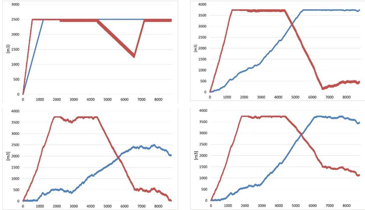
Fig. A3. Evolution of volume in the storage water tank throughout the year. The blue line indicates the volume considering a constant demand; the red line indicates the volume considering variable demand. From top to bottom and left to right: Case 0, Case 1, Case 2, and Case 3.
