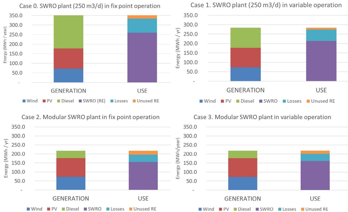
Fig. 7. Charts of the annual energy balance for each case (units: MWh/year).
