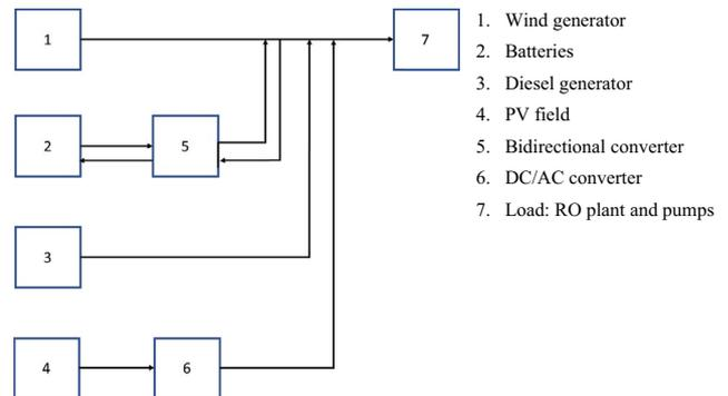
Fig. A2. Diagram of the main components of the system.
