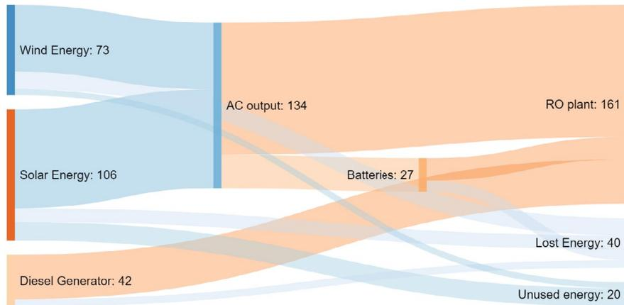
Fig. 5. Illustrations of power flows. Case of generation > demand (Figures in MWh/a).
