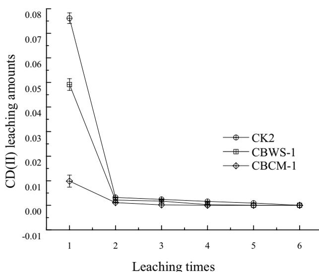
Fig. 4. Cd(II) leaching characteristics in the contaminated tea garden soils amended with biochar.
