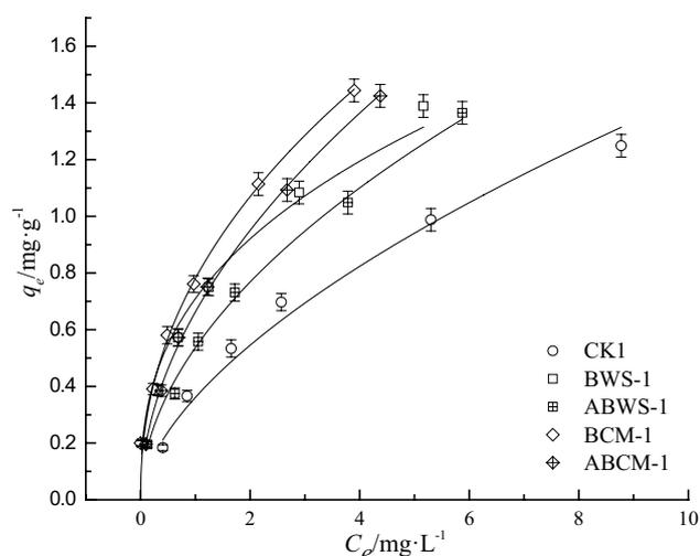
Fig. 2. Cd(II) adsorption isotherms in tea garden soils amended with aged biochar.
