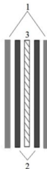
Fig. 1. Schematics picture of the CDI electrode assembly. 1 - graphite current collectors, 2 - AC electrodes, 3 - mosaic membrane.
