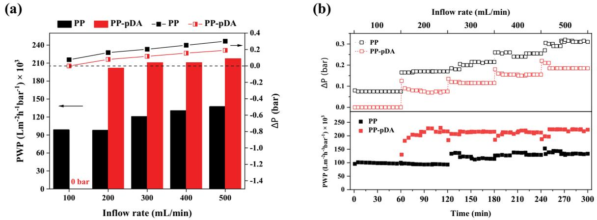
Fig. 6. PWP and ΔP (pressure differences) result of filter media (a) depending on their inflow rate changes and (b) using a stepping method by changing the inflow conditions every hour for 5 h.
