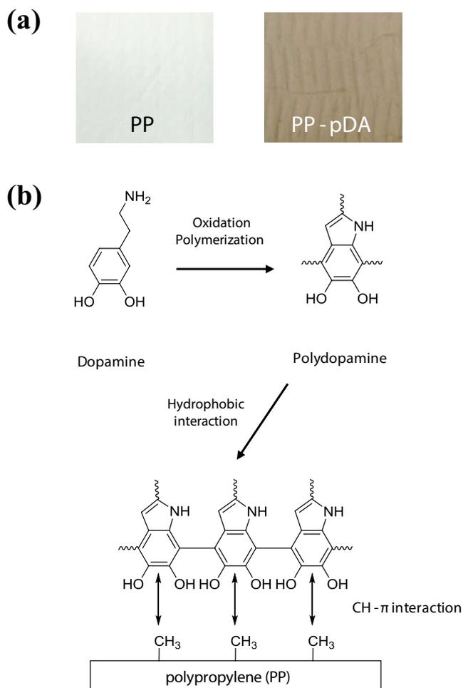
Fig. 3. (a) Digital images of filter media surfaces and (b) reaction scheme of oxidation polymerization and hydrophobic interaction between pDA and PP filter media.
