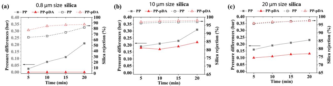
Fig. 7. Pressure differences and silica rejection comparison of filter media depending on the silica particle size: (a) 0.8, (b) 10, and (c) 20 μm.
