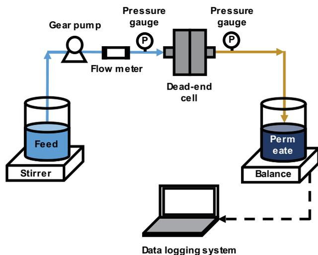
Fig. 2. Schematic diagram of the filtration system for filter media performance test.
