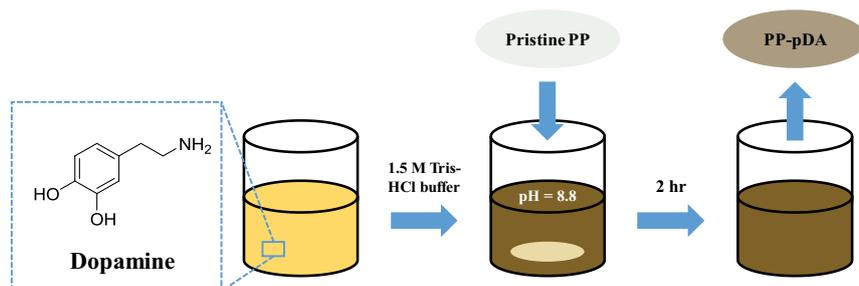
Fig. 1. Schematic description of pDA coating process of PP filter media.
