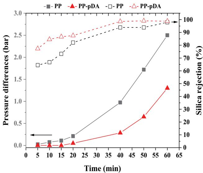
Fig. 8. Pressure differences and silica rejection trend of PP and PP-pDA filter media depending on time using 0.8 μm size of silica.
