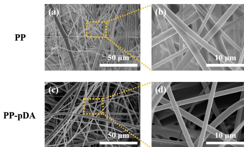
Fig. 4. SEM images of; (a, c) 1,000 $\times$  magnification and (b, d) 5,000 $\times$  magnification of PP and PP-pDA filter media, respectively.
