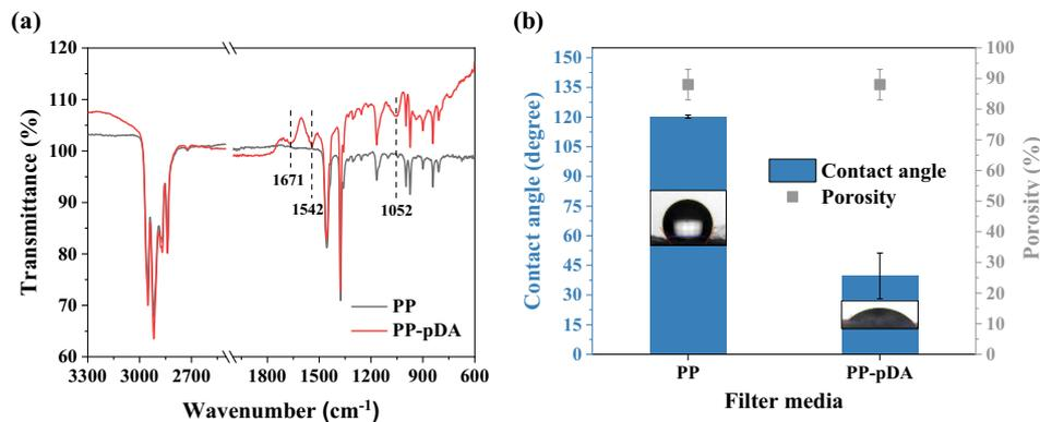
Fig. 5. (a) FTIR spectra and (b) water contact angle and porosity of PP and PP-pDA filter media.
