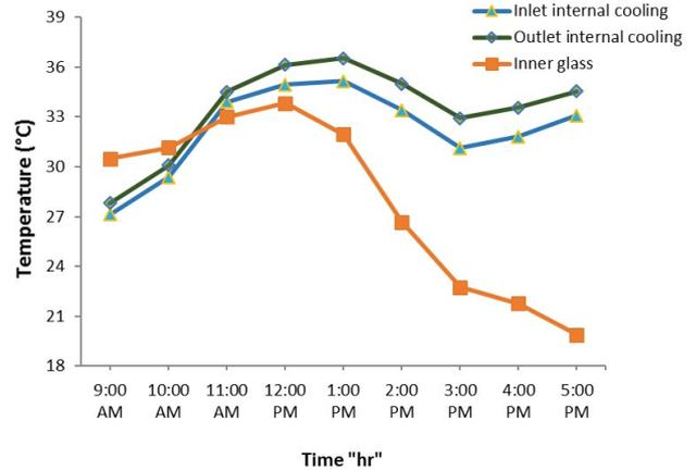
Fig. 12. Hourly variation of inlet and outlet temperatures of an internal cooling coil for conventional solar still using external film water cooling and an internal cooling coil (case 4).
