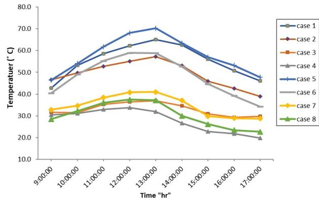
Fig. 8. Hourly variation of average glass temperatures of a solar still.
