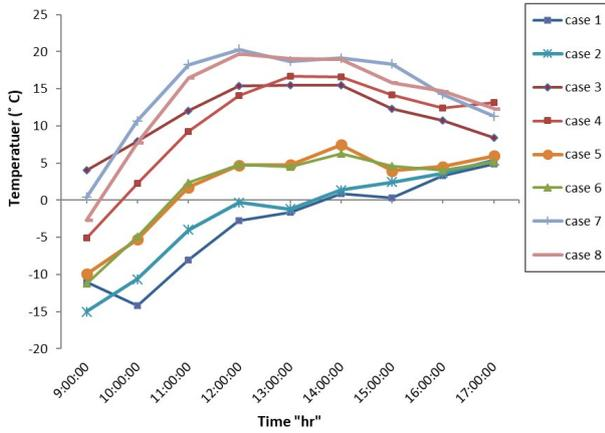
Fig. 10. Hourly variation of water – glass difference temperature of solar still.
