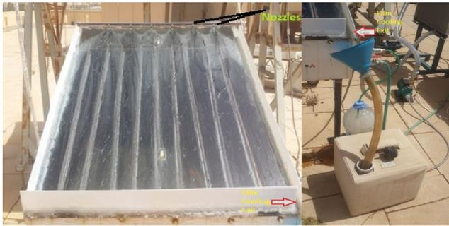
Fig. 5. Solar still system showing the external film water-cooling cycle.
