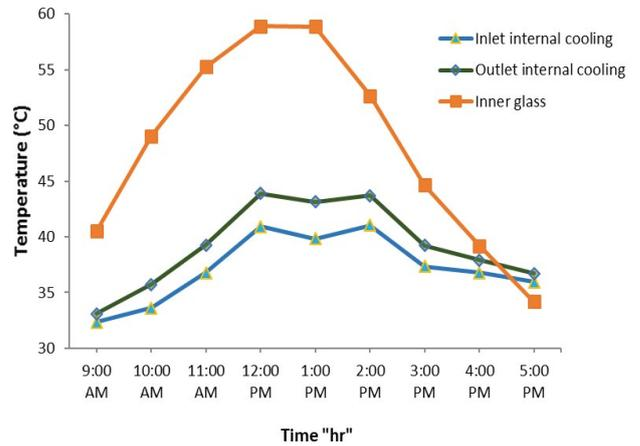
Fig. 13. Hourly variation of inlet and outlet temperatures of an internal cooling coil for a conventional solar still using parabolic trough heating and an internal cooling coil (case 6).
