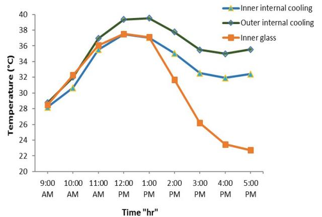
Fig. 14. Hourly variation of inlet and outlet internal cooling coil temperatures for a conventional solar still using parabolic trough heating along with internal and external cooling (case 8).
