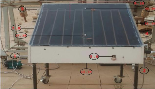
Fig. 1. Single solar still and thermocouples location numbers.
