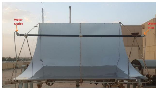
Fig. 4. Solar parabolic trough with iron pipe fixed on-axis line.
