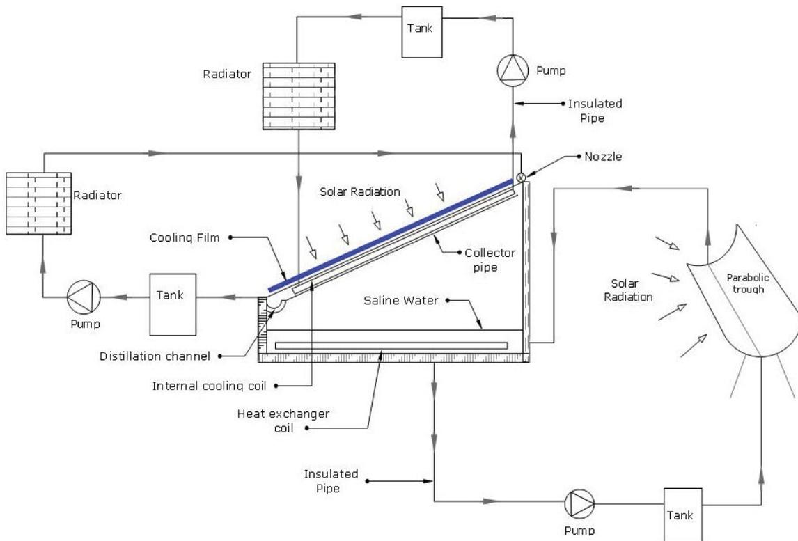
Fig. 6. Schematic diagram of the solar still system showing the internal cooling coil, external cooling, and parabolic trough loops.
