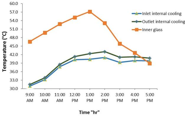
Fig. 11. Hourly variation of inlet and outlet temperatures of an internal cooling coil for a conventional solar still using an internal cooling coil (case 2).
