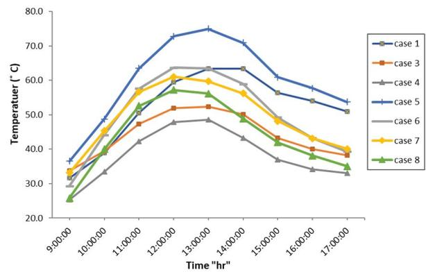
Fig. 9. Hourly variation of water temperatures in basin.
