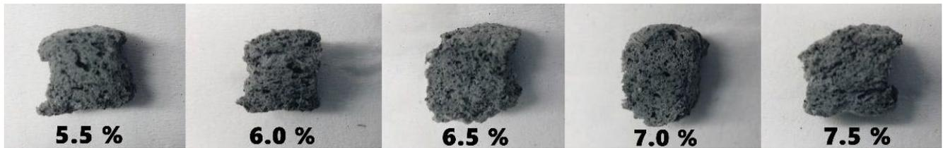
Fig. 1. LNR foam with different concentration of crosslinker (w/w %) to LNR.
