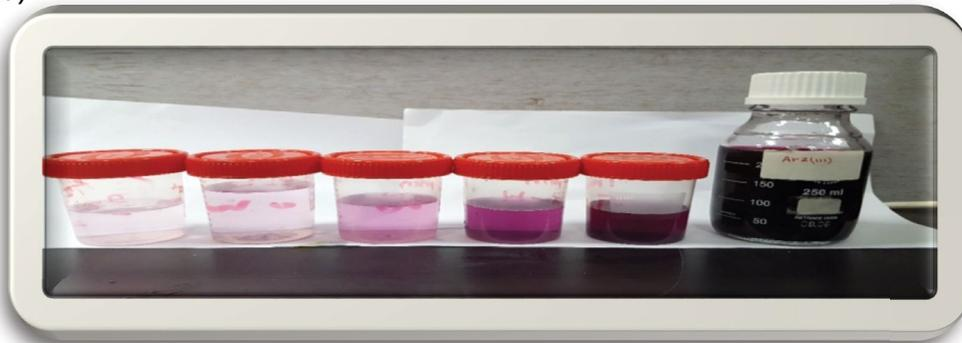
Figs. 2a and b. Picture of MB and arsenazo III dye after degradation at various times.
