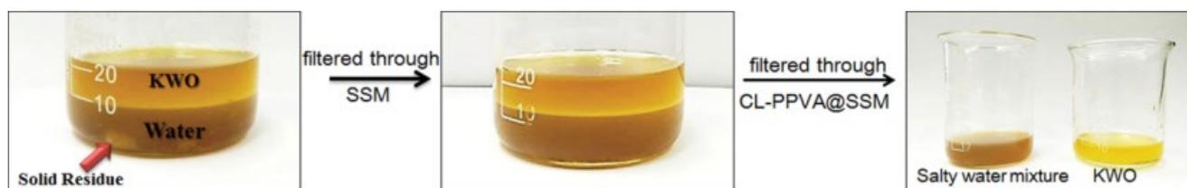
Fig. 14. Collection process of kitchen waste oil from catering trade by CL-PPVA@SSM.
