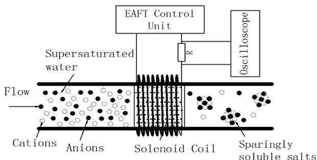
Fig. 2. Schematic diagram of the experimental device.
