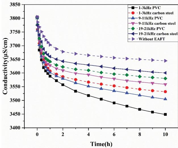
Fig. 4. Variation of conductivity with time under different frequencies.
