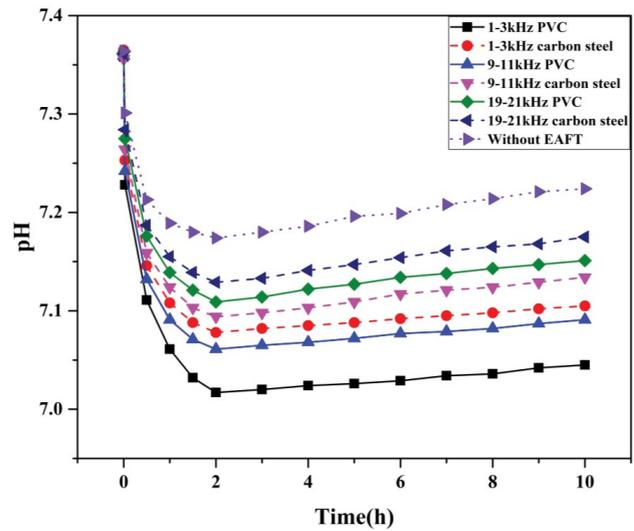
Fig. 5. Variation of pH with time under different frequencies.
