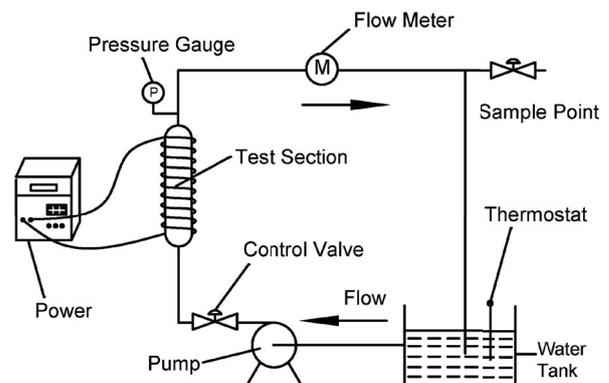
Fig. 3. Schematic diagram of the fouling test facility in the present study.
