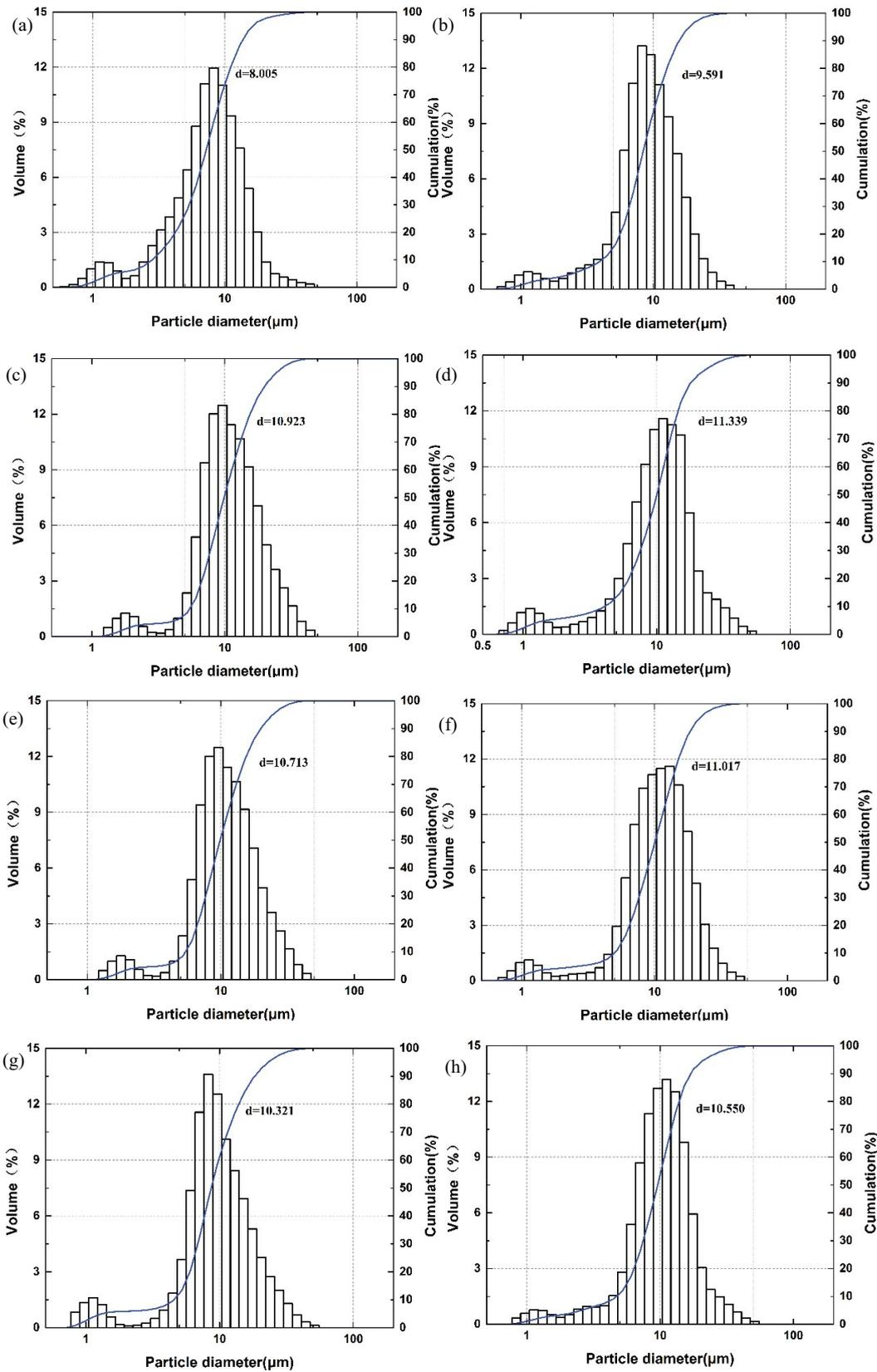
Fig. 7. Particle diameter. (a) Initial particle diameter, (b) without EAFT, (c) sweep frequency of 1–3 kHz in carbon steel pipe, (d) sweep frequency of 1–3 kHz in PVC pipe, (e) sweep frequency of 9–11 kHz in the carbon steel pipe, (f) sweep frequency of 9–11 kHz in the PVC pipe, (g) sweep frequency of 19–21 kHz in the carbon steel pipe, and (h) sweep frequency of 19–21 kHz in the PVC pipe.
