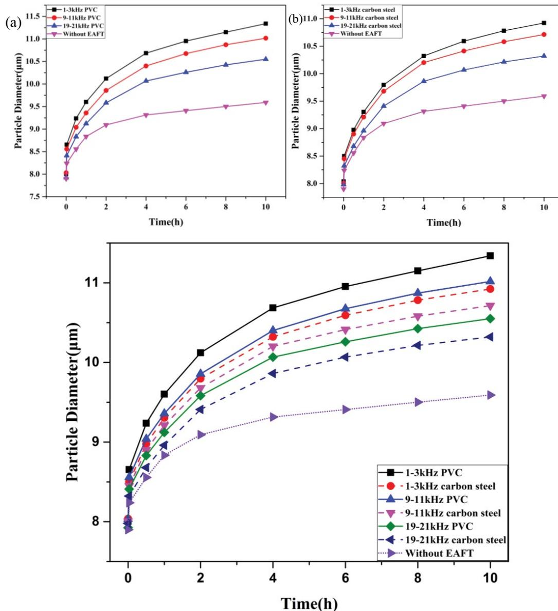
Fig. 6. Variation of average particle diameter with time under different frequencies. (a) Variation of average particle diameter with time in the PVC pipe under different frequencies and (b) variation of average particle diameter with time in the carbon steel pipe under different frequencies.
