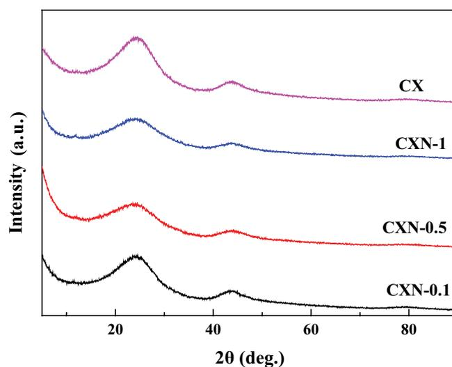
Fig. 3. XRD patterns of N-doped carbon xerogels.
