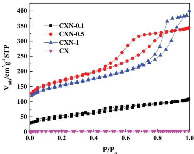
Fig. 1. Nitrogen adsorption-desorption isotherms for carbon xerogels.
