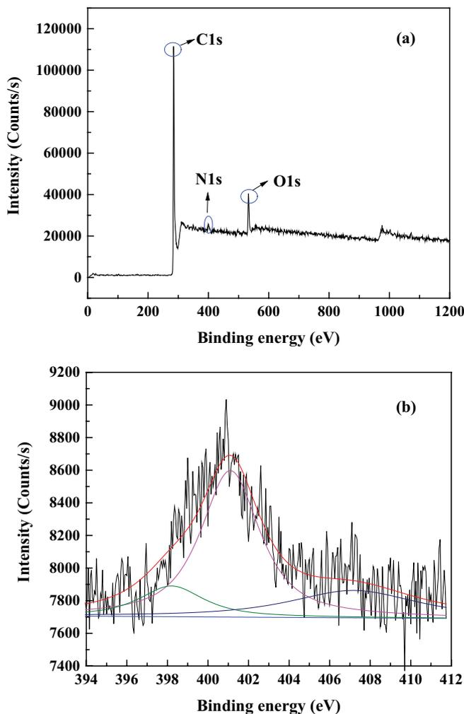
Fig. 2. XPS spectra of (a) survey scan and (b) N1s for CXN-1.
