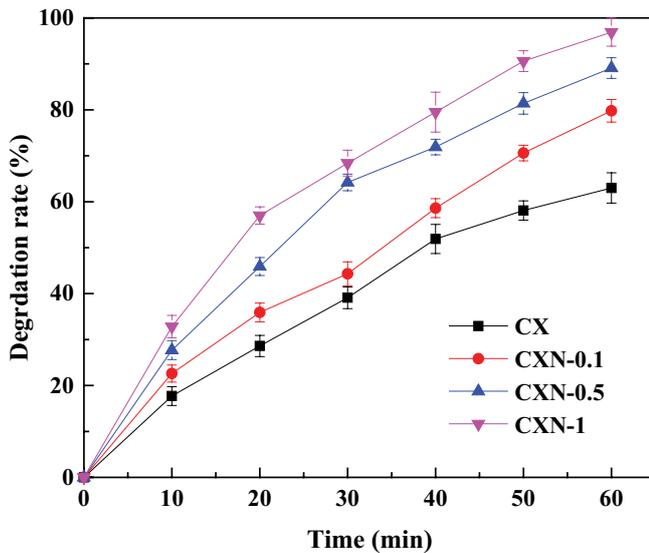
Fig. 5. Electro-catalytic degradation of CTRX by carbon xerogel anodes.
