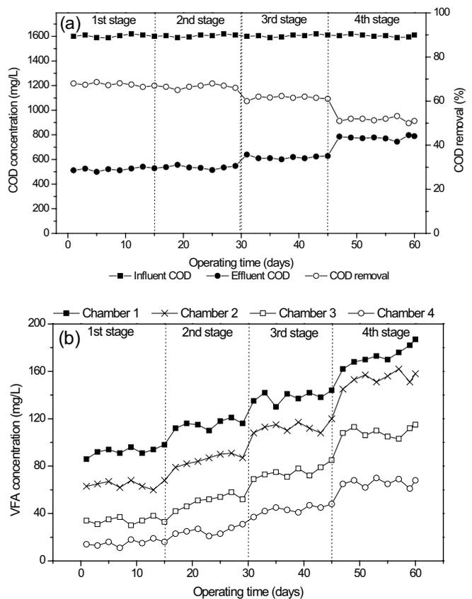
Fig. 4. Profile of COD removal (a) and VFA production (b) in each chamber during the experimental processes of ABR.
