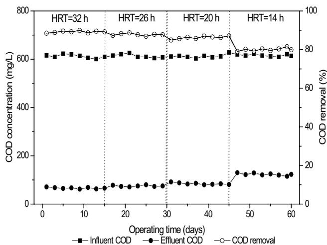
Fig. 5. Influent and effluent COD concentrations and COD removal during the 60 d operation of the BCO system.
