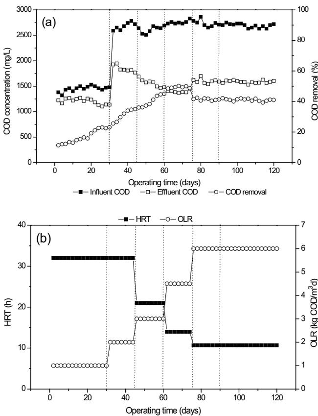
Fig. 3. (a) EGSB COD treatment efficiency and (b) corresponding HRT and OLR.
