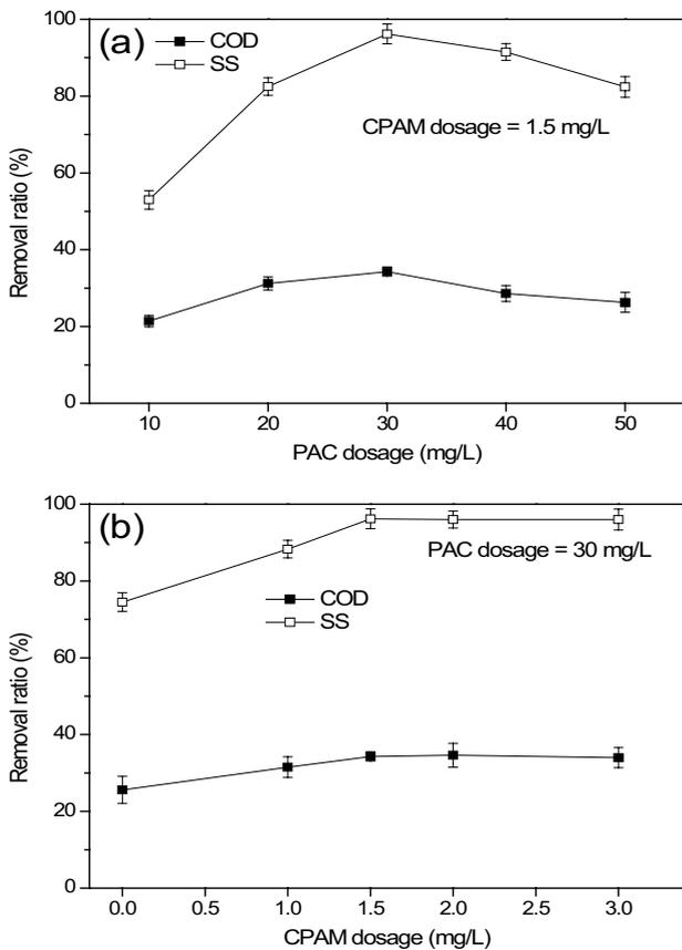
Fig. 2. Effect of (a) PAC dosage and (b) CPAM dosage on COD and SS removal during coagulation tests.
