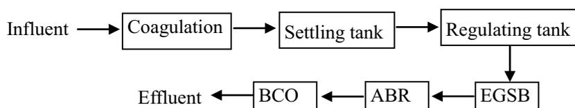
Fig. 1. Schematic flow chart of the PPW treatment system.
