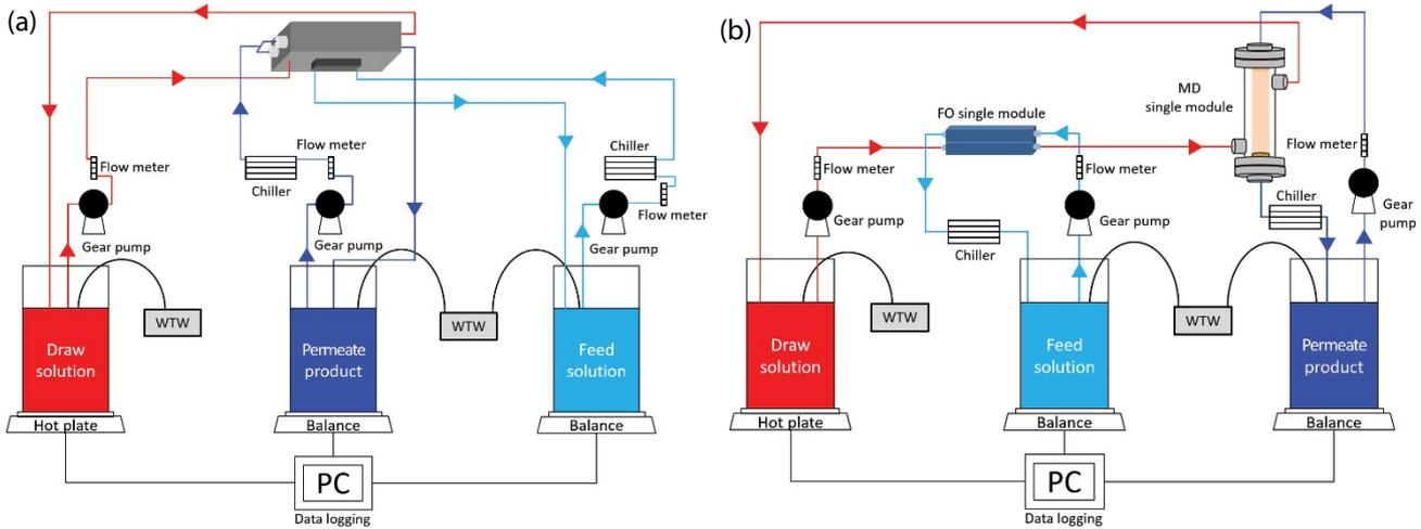
Fig. 1. Schematic diagrams of each system. (a) Integrated module system and (b) single module hybrid system.
