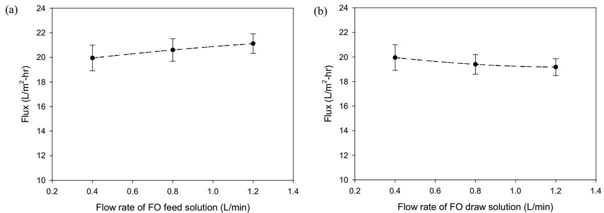
Fig. 3. Effect of flow rate in the FO process in the integrated FO-MD module. (a) Flow rate of feed solution and (b) flow rate of draw solution.
