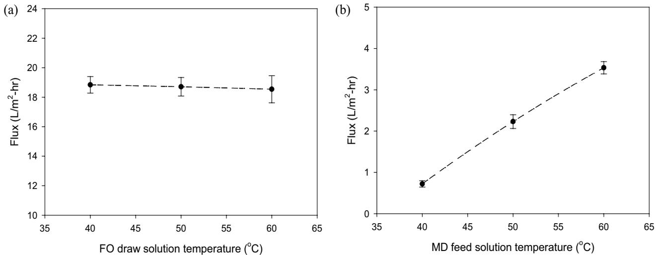
Fig. 5. Effect of solution temperature in the FO process in the integrated FO-MD module. (a) Draw solution temperature and (b) feed solution temperature.
