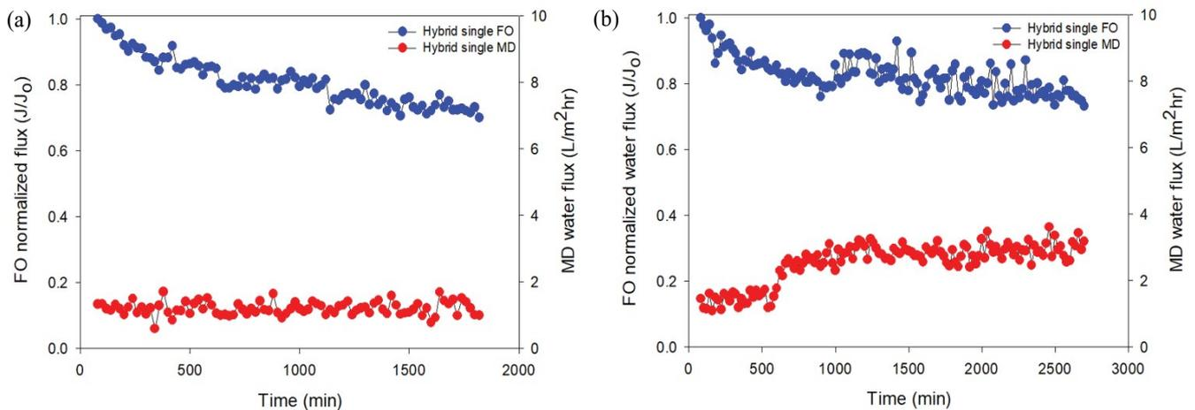
Fig. 6. Flux behaviors in the FO-MD hybrid system using separate FO and MD modules. (a) Constant temperature of the draw solution at 50°C and (b) adjustment of the temperature of the draw solution between 50°C and 60°C.
