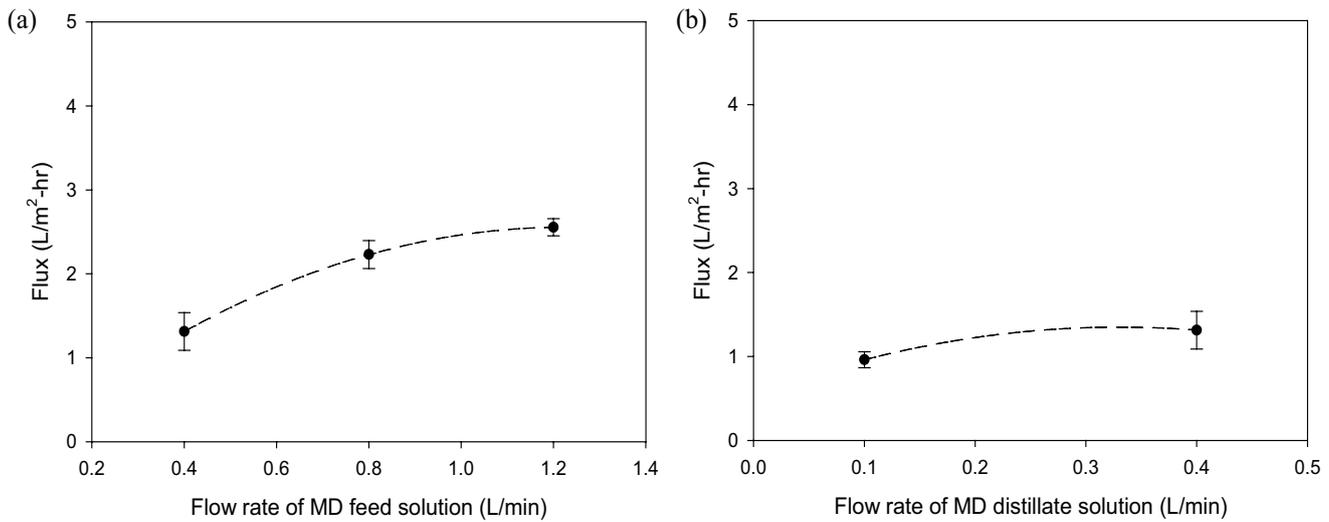
Fig. 4. Effect of flow rate in the hollow-fiber DCMD process in the integrated FO-MD module. (a) Flow rate of feed solution and (b) flow rate of distillate solution.
