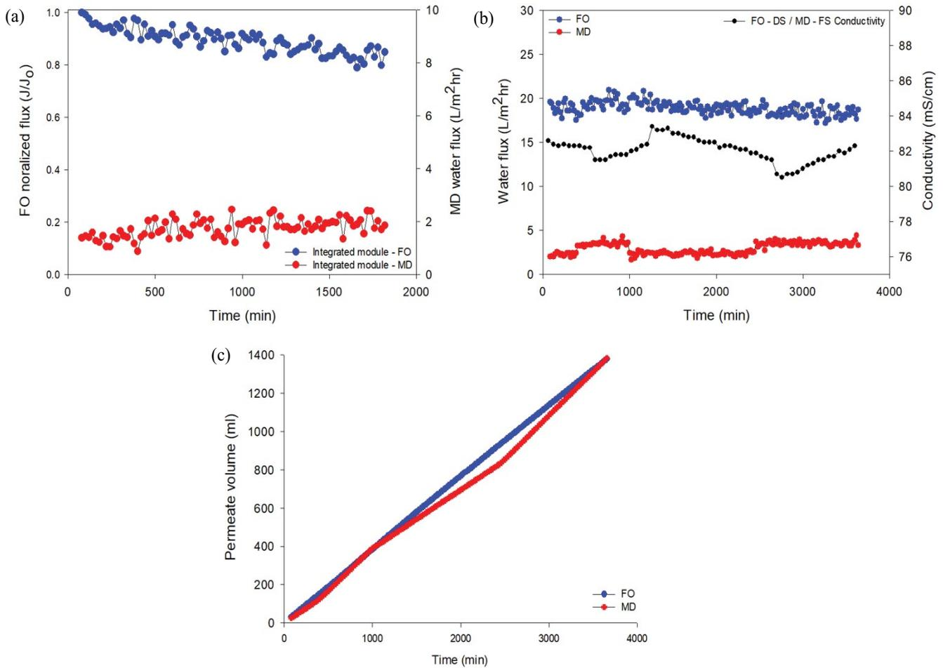
Fig. 7. Flux behaviors in the FO-MD hybrid system using an integrated module. (a) Constant temperature of the draw solution at 50°C, (b) adjustment of the temperature of the draw solution between 50°C and 60°C, and (c) comparison of the permeate volumes from FO and MD membranes.
