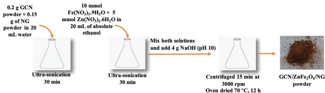
Fig. 2. Schematic illustration of GCN/ZnFe<sub>2</sub>O<sub>4</sub>/NG synthesis. (Similar method was used for the fabrication of GCN/CoFe<sub>2</sub>O<sub>4</sub>/NG, 5 mmol of Co(NO<sub>3</sub>)<sub>2</sub>·6H<sub>2</sub>O was added instead of Zn(NO<sub>3</sub>)<sub>2</sub>·6H<sub>2</sub>O).
