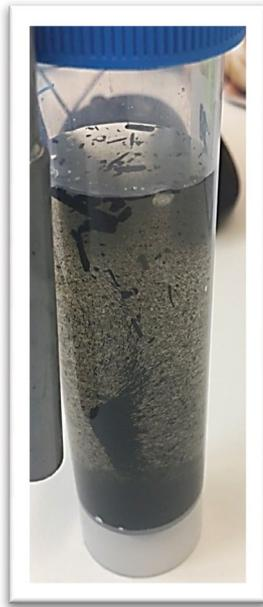
Fig. 11. The engineered Fe-biochar sample (BC-C), showing magnetic properties by attraction to the permanent magnet.
