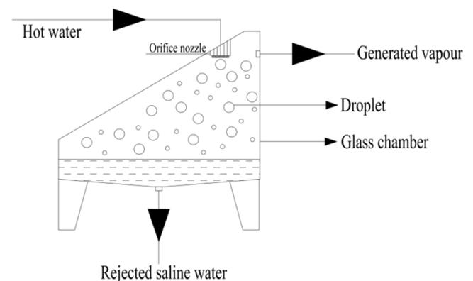
Fig. 1. Vapor production chamber in the system.
