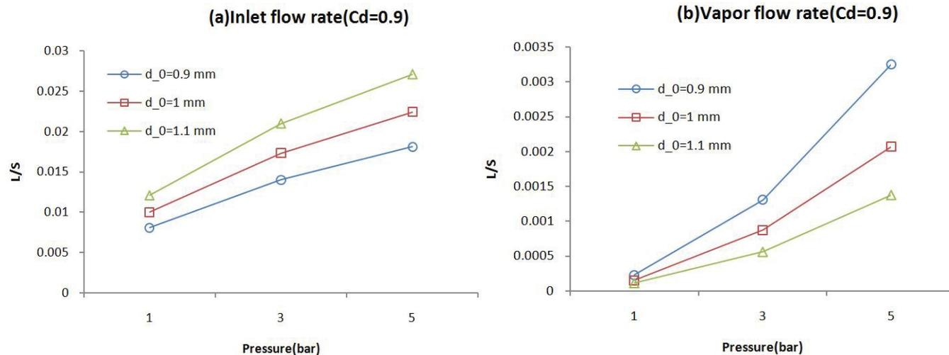
Fig. 10. Effect of outlet diameter of nozzle on flow rate of (a) sprayed inlet water and (b) produced vapor.
