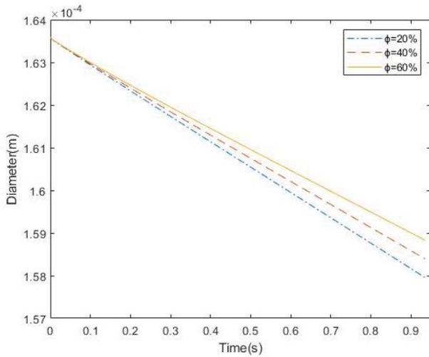
Fig. 9. Reduction of the droplets' diameter at the injection pressure of 3 bar.
