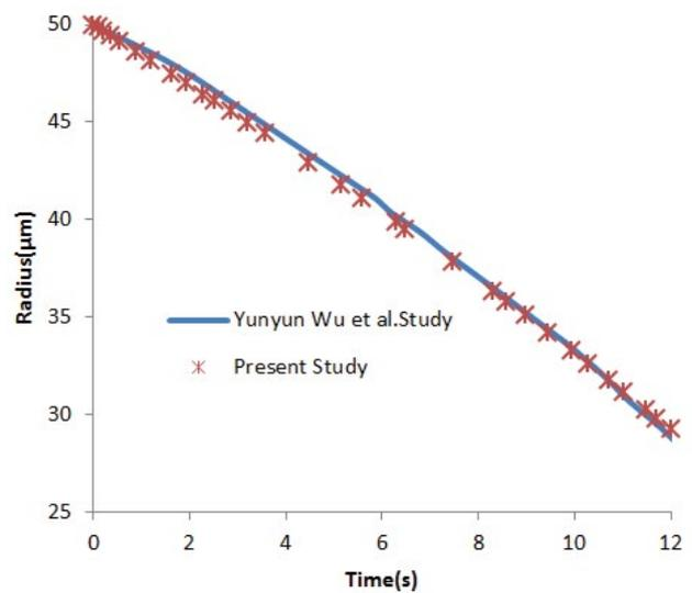
Fig. 4. Verification of the diameter reduction in relative humidity of 20% and surrounding temperature of 5°C.
