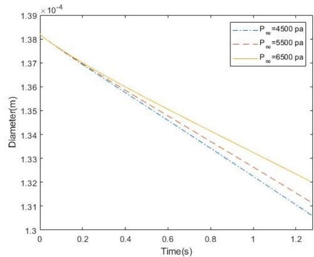
Fig. 8. Reduction of the droplets' diameter at the injection pressure of 5 bar.
