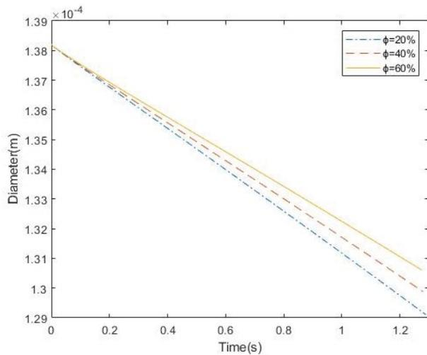
Fig. 6. Reduction of the droplets' diameter at nozzle outlet diameter of 0.9 mm.
