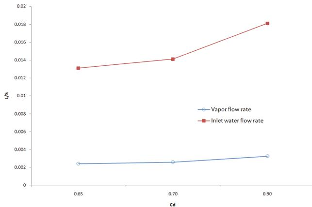
Fig. 11. Effect of nozzle type on flow rate of sprayed inlet water and produced vapor.
