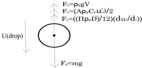
Fig. 2. Forces on a droplet in downward spraying system.
