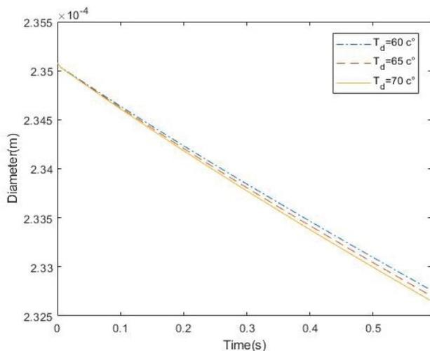
Fig. 7. Reduction of the droplets' diameter at the injection pressure of 1 bar.
