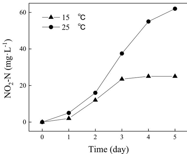
Fig. 8. Changes of NO<sub>2</sub>-N concentrations from different groups with different temperatures.
