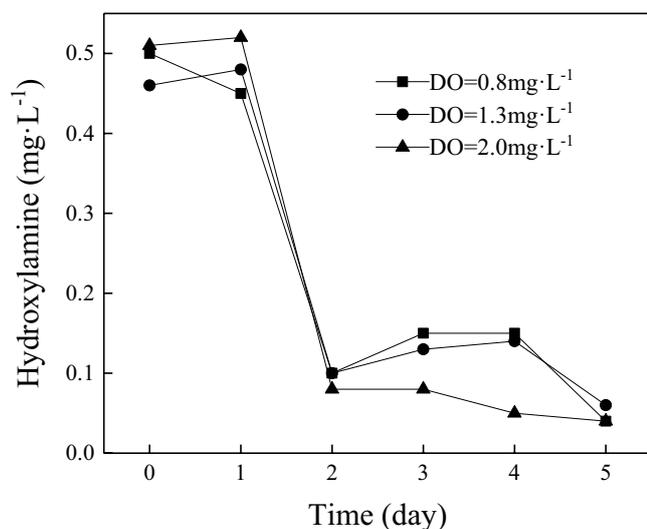
Fig. 6. Changes of hydroxylamine concentrations from different groups with different DO contents.
