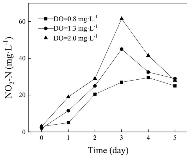
Fig. 5. Changes of NO<sub>2</sub>-N concentrations from different groups with different DO contents.
