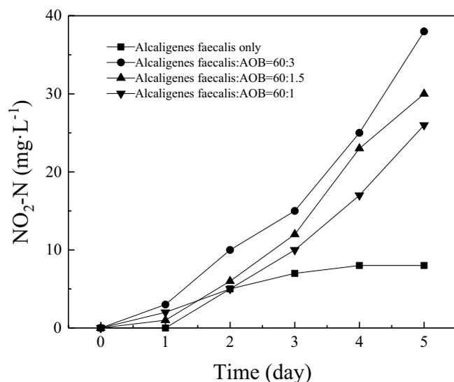
Fig. 11. Changes of  $\text{NO}_2\text{-N}$  concentrations from different groups with different *A. faecalis*/AOB ratios.
