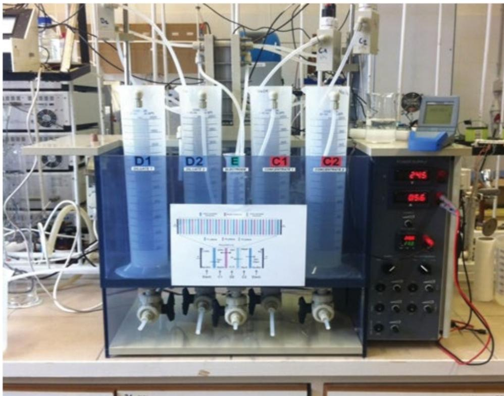
Fig. 2. Image of the multifunctional P EDR-Z/4x electrodiolysis equipment.
