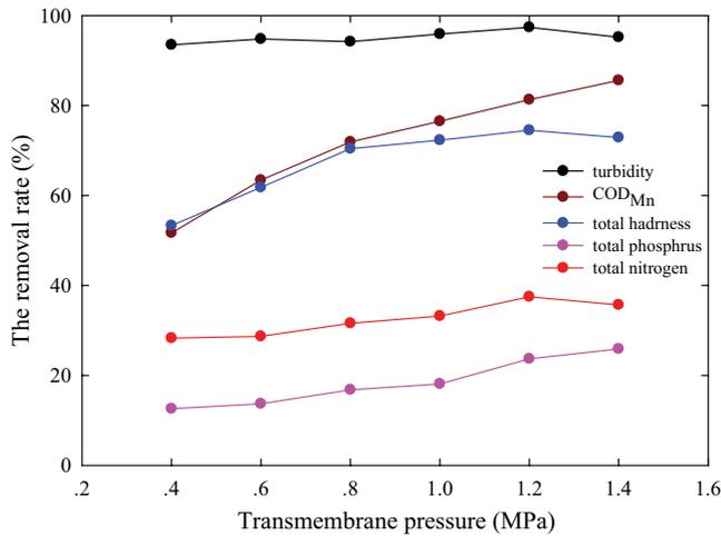
Fig. 2. Removal rate with transmembrane pressure (flow rate 30 L/min, 25°C ± 1°C, operation time 24 h).
