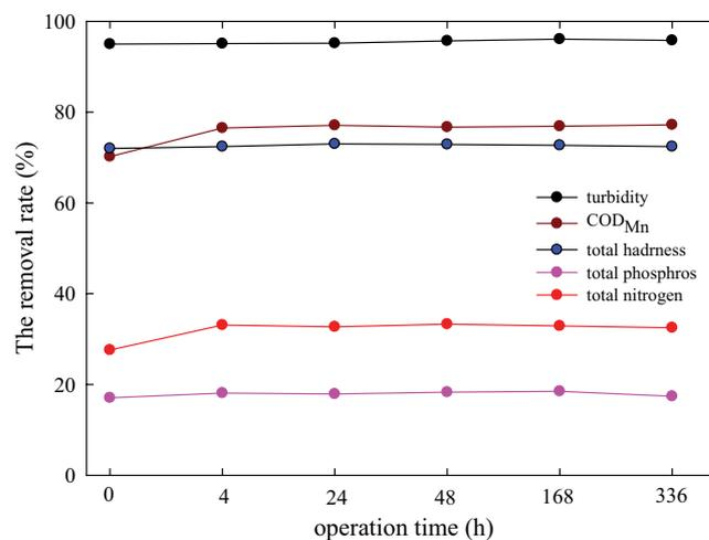
Fig. 7. Removal variation with operation time ( $\Delta P = 1.0$  MPa, flow rate 30 L/min,  $25^{\circ}\text{C} \pm 1^{\circ}\text{C}$ ).
