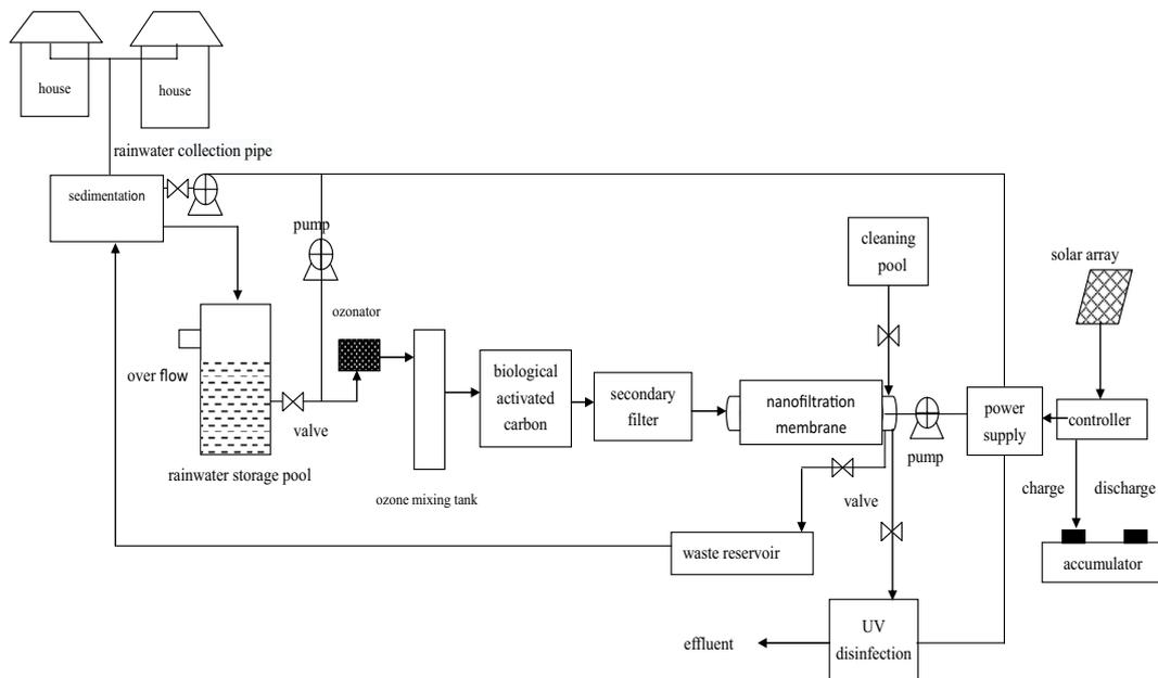
Fig. 1. Schematic diagram of the experimental equipment.
