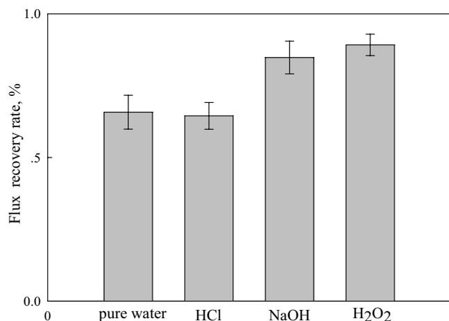
Fig. 8. Membrane flux recovery after chemical cleaning ( $\Delta P = 1.0$  MPa, flow rate 30 L/min,  $25^\circ\text{C} \pm 1^\circ\text{C}$ ).
