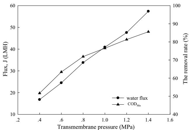
Fig. 3. Variation of flux and COD<sub>Mn</sub> removal rate with transmembrane pressure (flow rate 30 L/min, 25°C ± 1°C, operation time 24 h).
