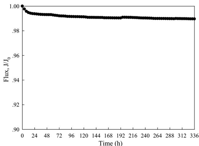
Fig. 6. Variation of flux with operation time ( $\Delta P = 1.0$  MPa, flow rate 30 L/min,  $25^{\circ}\text{C} \pm 1^{\circ}\text{C}$ ).
