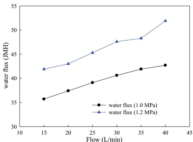
Fig. 5. Variation of flux with the different flow ( $25^{\circ}\text{C} \pm 1^{\circ}\text{C}$ ).
