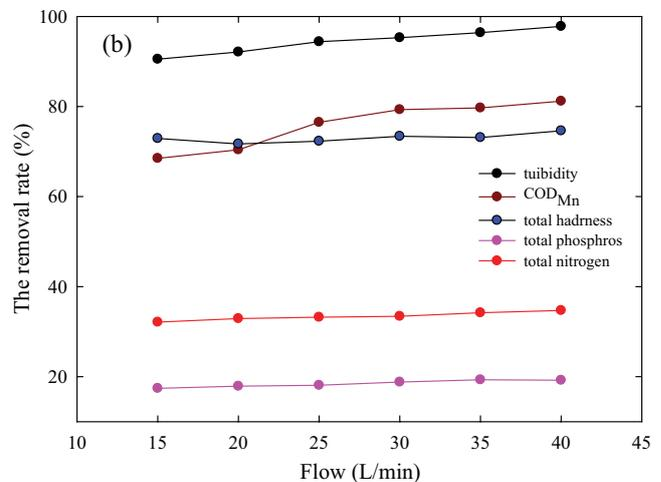
Fig. 4. Removal rates of contaminants under different flows at 25°C ± 1°C with 24 h (a) ΔP = 1.0 MPa and (b) ΔP = 1.2 MPa.
