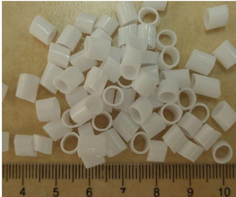
Fig. S2. Propylene plastic media used in the absorption column.
