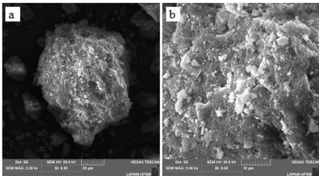
Fig. 4. SEM image of the sludge at 2,000 $\times$  magnification (a) and 5,000 $\times$  magnification (b).
