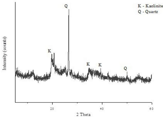
Fig. 2. X-Ray diffractogram of WTP sludge.
