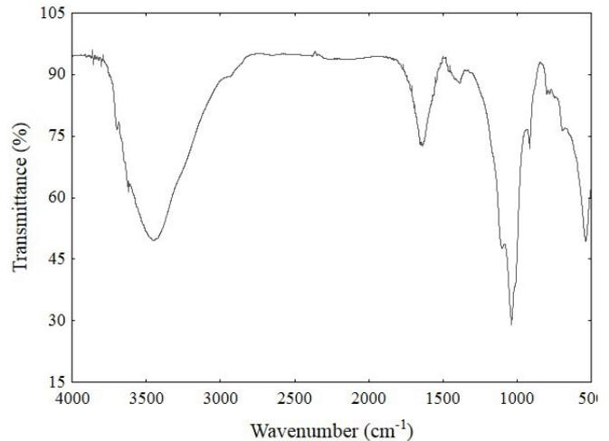
Fig. 3. FT-IR spectrum of WTP sludge.
