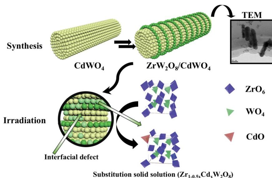
Fig. 1. Schematic diagram of the synthesis process and TEM diagram of the final product.
