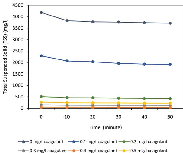
Fig. 7. Reduction of TSS in wastewater after adding coagulant and processed using DBDi technology.
