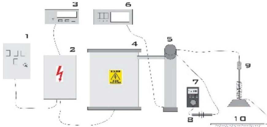
Fig. 1. DBD ionization reactor (1) AC power supply, (2) regulator, (3) operating terminal, (4) step-up transformer, (5) capacitors, (6) digital measuring instrument (7) multimeter, (8) probe, (9) DBDI reactor, and (10) ground.
