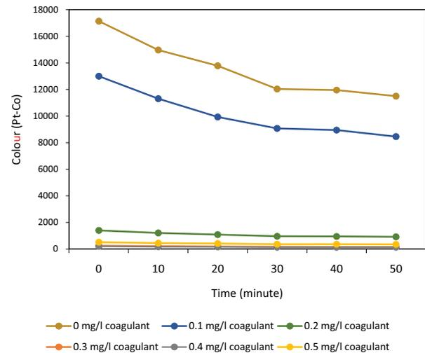
Fig. 8. Reduction of color in wastewater after adding coagulant and processed using DBDi technology.
