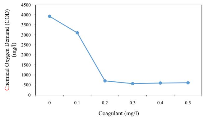
Fig. 2. Reduction of COD by coagulant.
