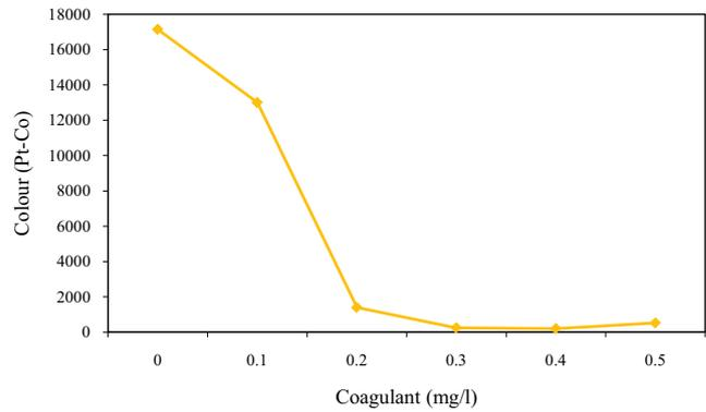
Fig. 4. Reduction of color by coagulant.
