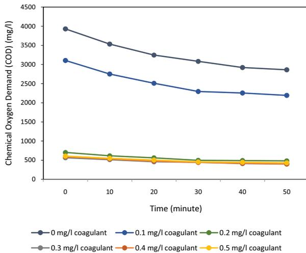
Fig. 6. Reduction of COD concentration after adding coagulant and processed using DBDi technology.
