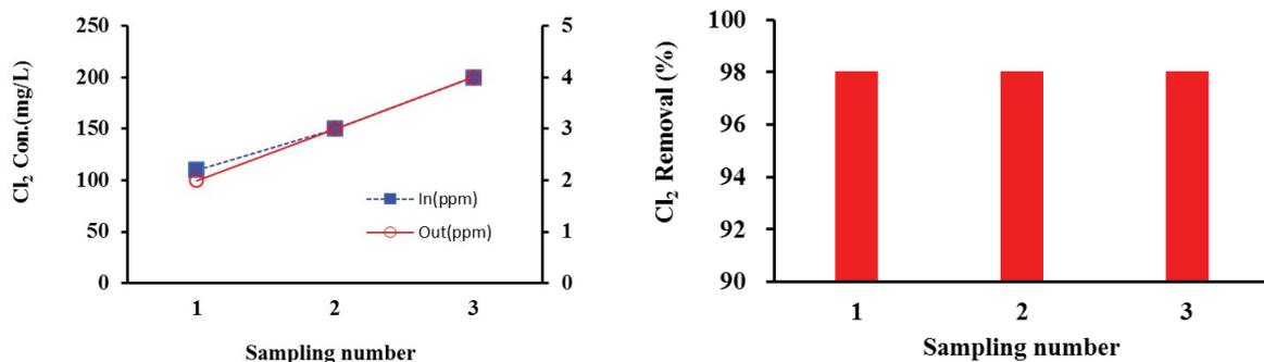
Fig. 7. Variation of influent and effluent chlorine concentration and removal efficiency with the function of sampling times chlorine gas treatment.
