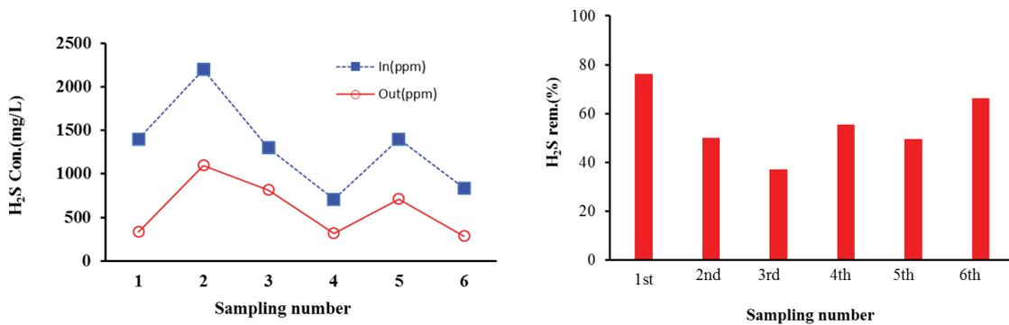
Fig. 6. Variation of influent and effluent  $H_2S$  concentration and removal efficiency with the function of sampling times.
