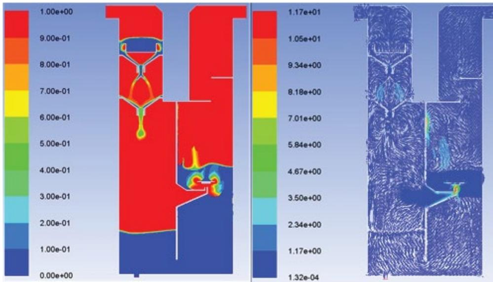
Fig. 3. CFD analysis during the operation: air and water are fully mixed (left), then the velocity is rapidly increased through the collapsing of the atomizing devices.
