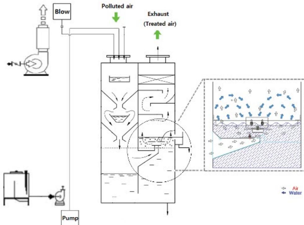
Fig. 1. Schematic of dip injection wet scrubber generating fine bubbles through the air atomizer.
