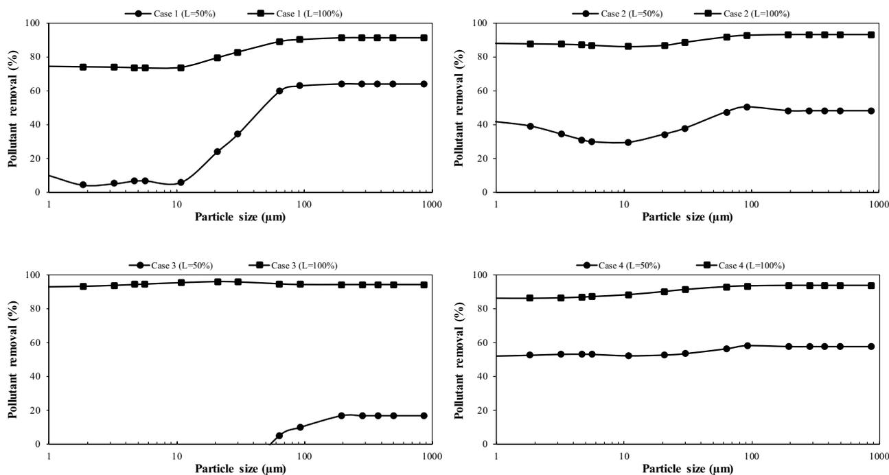
Fig. 6. Removal of varying particle sizes with respect to facility length.
