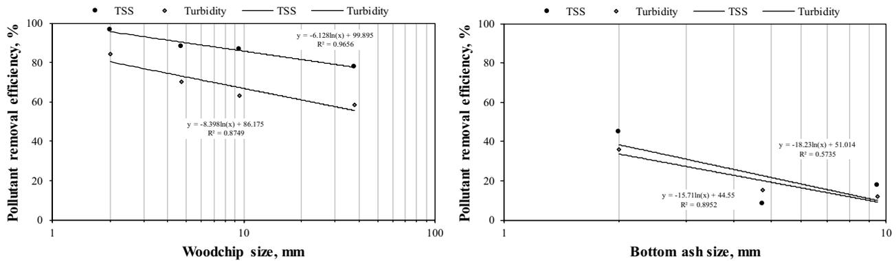
Fig. 4. Changes in pollutant removal efficiency at varying filter media sizes.
