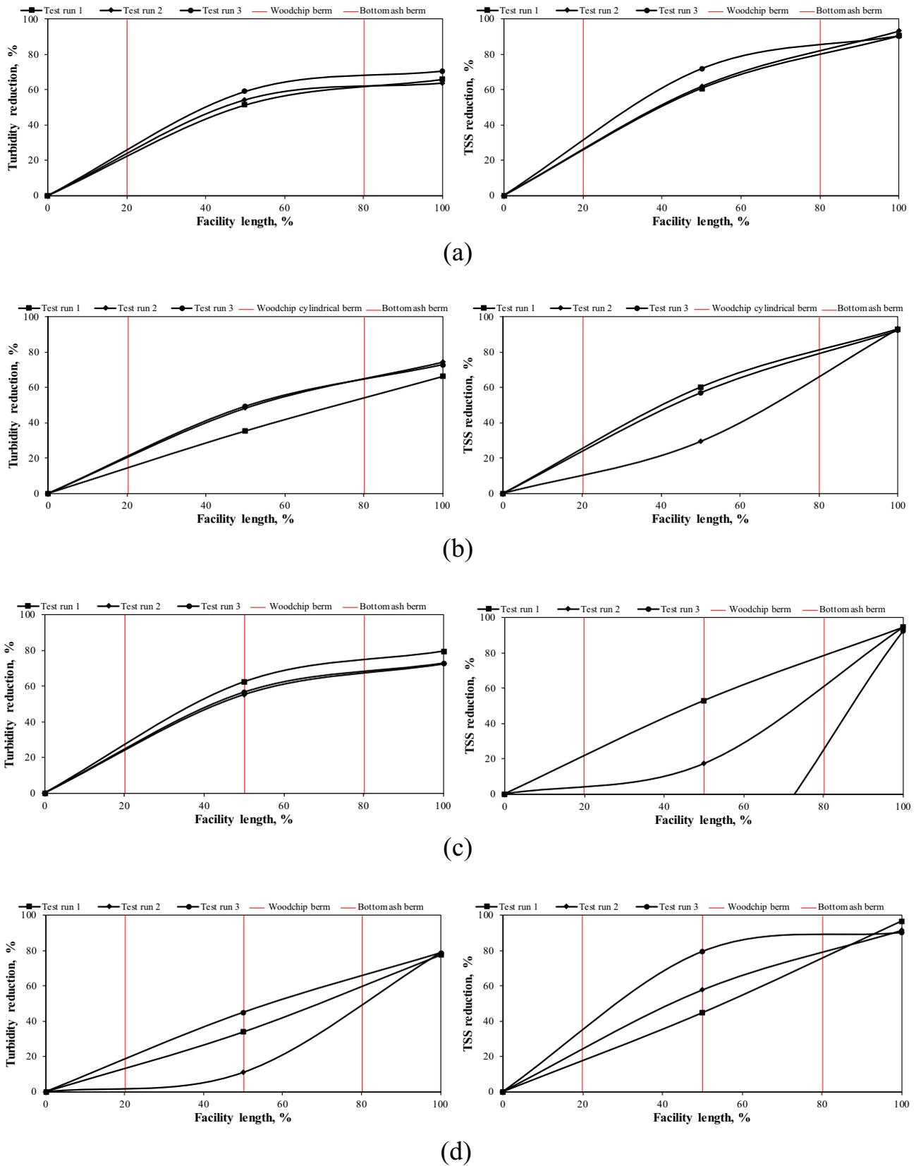
Fig. 5. Changes in pollutant concentration with respect to facility length (a) case 1, (b) case 2, (c) case 3, and (d) case 4.
