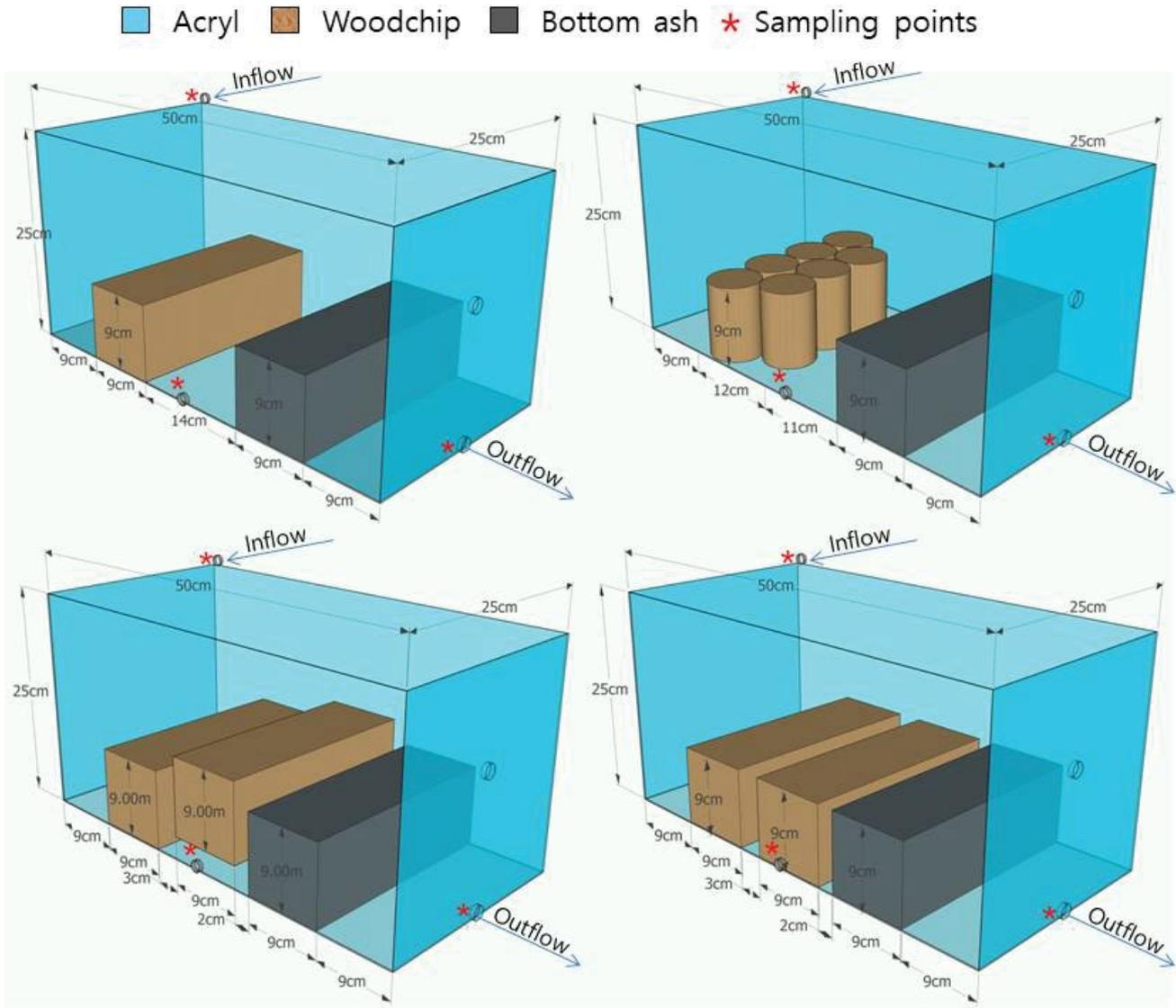
Fig. 2. Design configurations of pilot-scale facilities.
