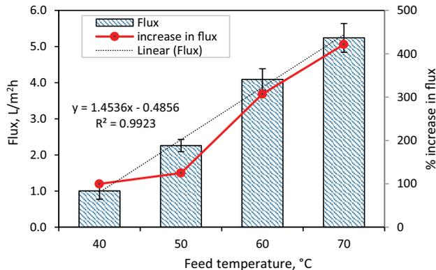
Fig. 2. Water flux at different temperatures under the condition: feed TDS of 5,000 mg/L, cooling stream temperature of  $28^{\circ}\text{C} \pm 1^{\circ}\text{C}$ .
