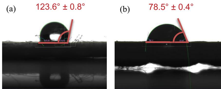
Fig. 5. Contact angles of (a) pristine membrane and (b) fouled membrane after 2 months of operation (the feed temperature of 60°C, and cooling stream temperature of 28°C ± 1°C).
