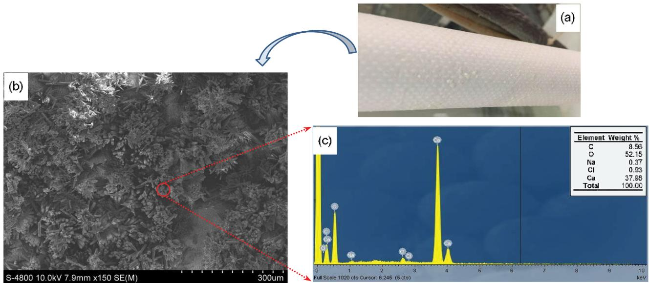
Fig. 6. Fouled membrane after long-term operation under conditions (feed TDS of 30,000 mg/L, feed temperature of 60°C, and cooling stream temperature of 28°C ± 1°C). (a) Actual membrane surface scaling, (b) scanning electron microscopy (SEM), and (c) energy-dispersive X-ray spectroscopy (EDX).
