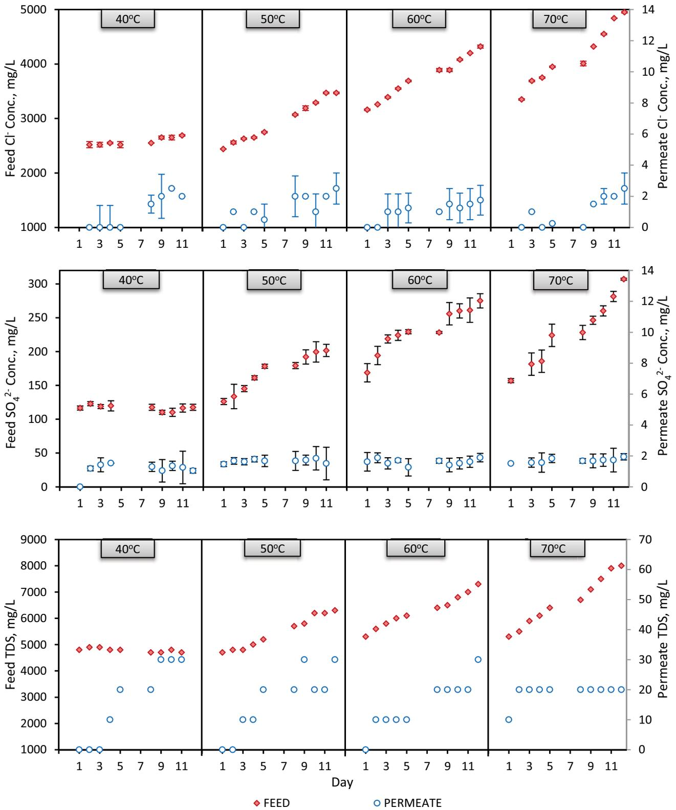
Fig. 3. TDS, chloride concentration, and sulfate concentration at different feed temperatures (40, 50, 60, and 70) another condition: the cooling stream temperature of 28°C ± 1°C.
