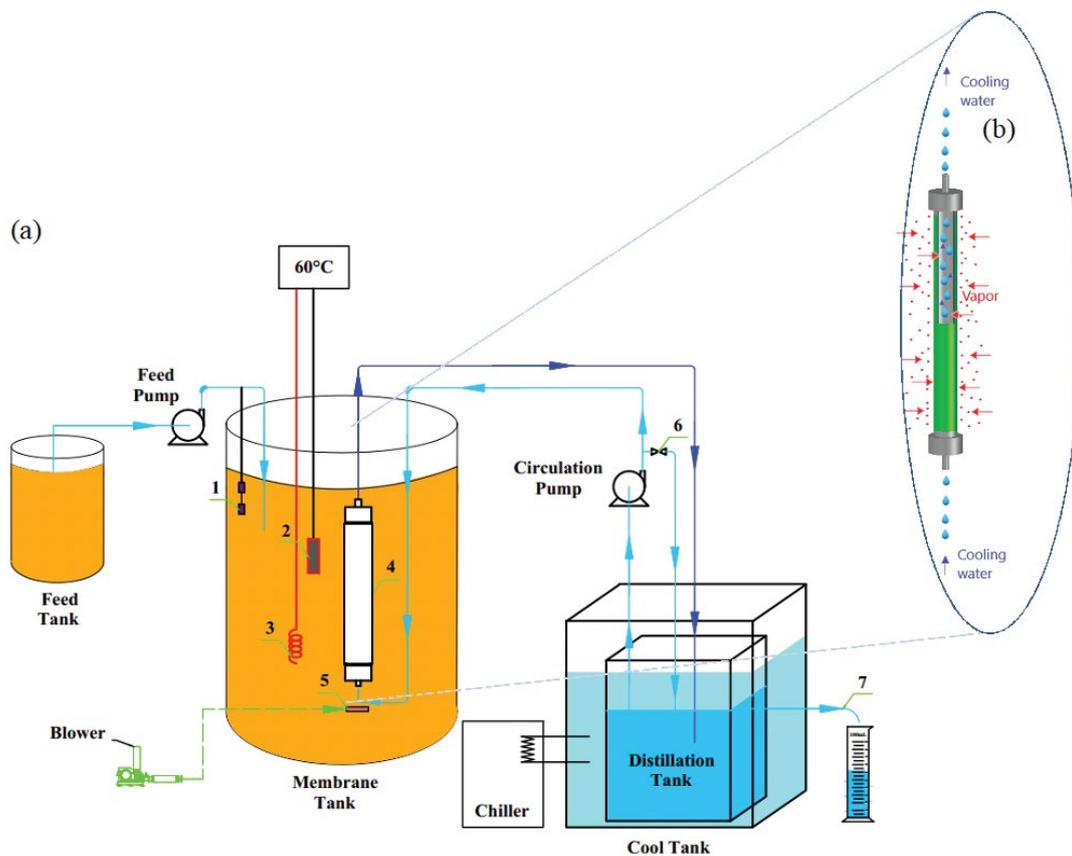
Fig. 1. (a) Schematic diagram of direct contact membrane distillation (DCMD) system and (b) principle of membrane module operation.
