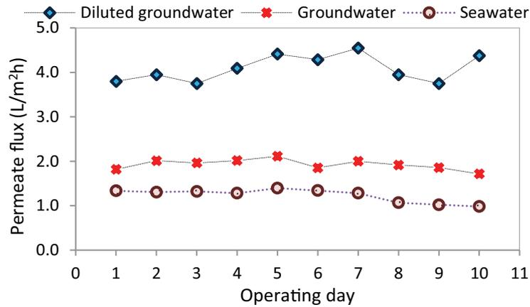
Fig. 4. Effect of feed TDS on permeate flux at a feed temperature of 60°C and cooling stream temperature of 28°C ± 1°C.
