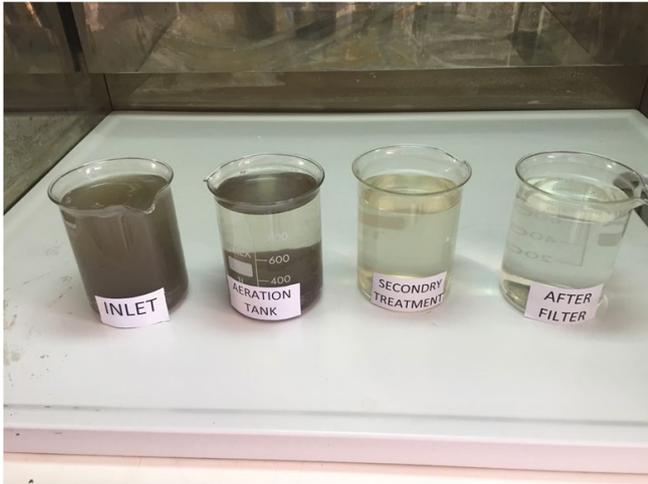
Fig. S2. Wastewater before and after treatment stages of TSTP.
