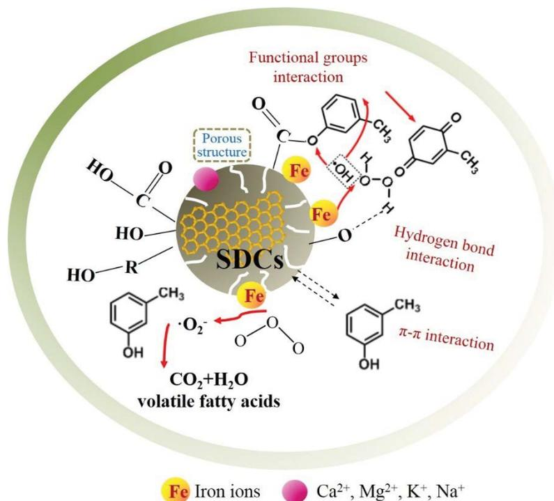
Fig. 3. Degradation of *m*-cresol with SDCs in CWPO and CWO by various mechanisms.
