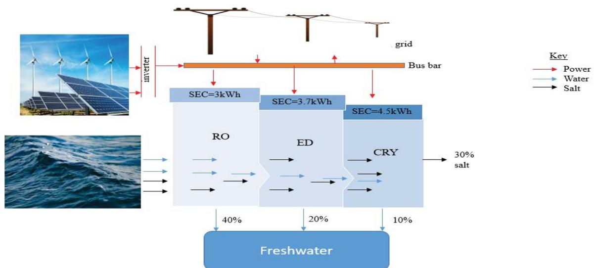
Fig. 1. Schematic diagram of combined desalination and brine treatment process.
