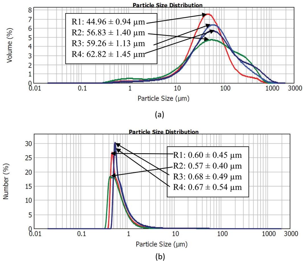
Fig. 3. (a) Microbial flocs size distribution of the different anaerobic membrane bioreactors added with different sizes of PAC in terms of volume and (b) number.
