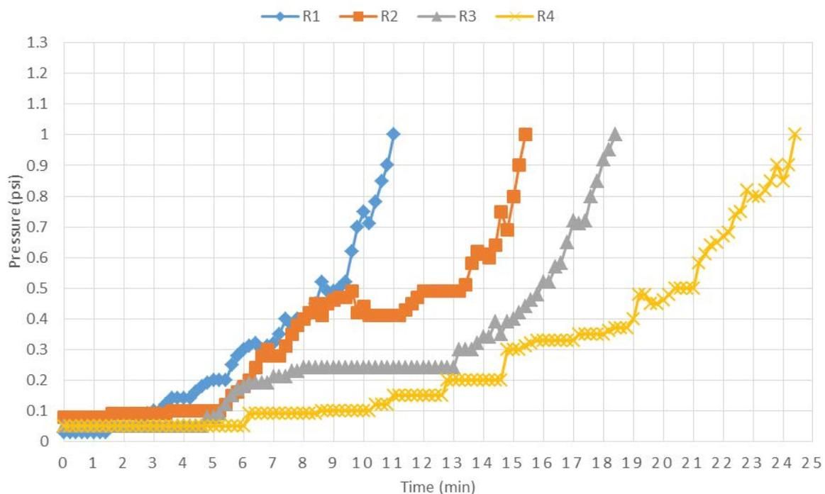
Fig. 2. Performance of membrane fouling control of different anaerobic membrane bioreactors added with different sizes of powdered activated carbon presented by the transmembrane pressure.
