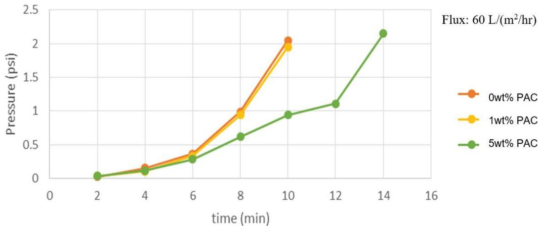
Fig. 4. Membrane fouling control performance of the different hybrid membranes incorporated with different PAC concentrations represented by the transmembrane pressure.
