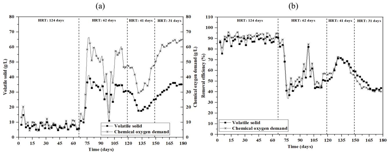
Fig. 5. (a) Variations and (b) removal efficiencies in terms of volatile solid and chemical oxygen demand in daily feeding mode's discharged effluent during operation under declined HRTs.
