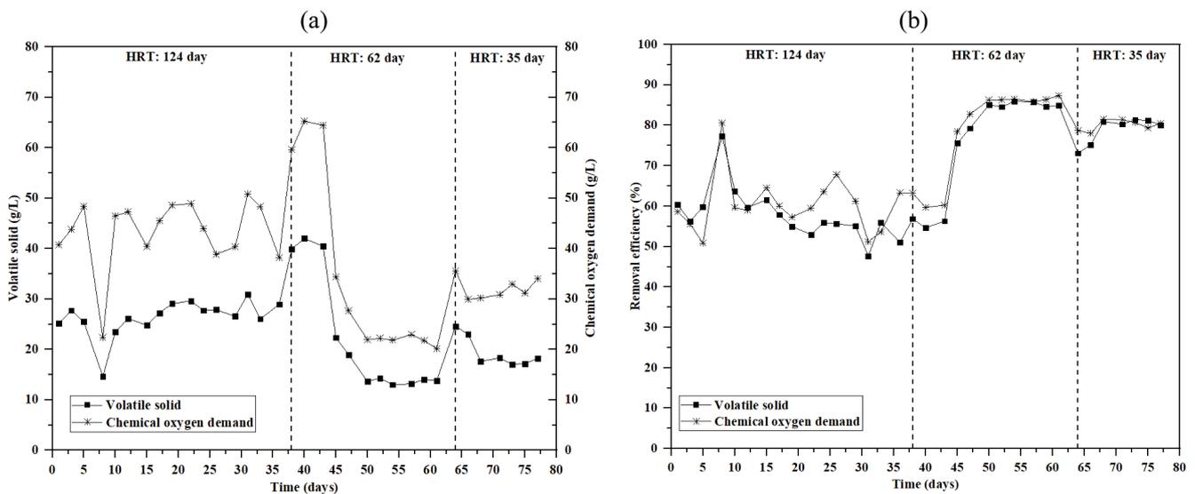
Fig. 6. (a) Variations and (b) removal efficiencies in terms of volatile solid and chemical oxygen demand in 3-times-per-week feeding mode's discharged effluent during operation under declined HRTs.
