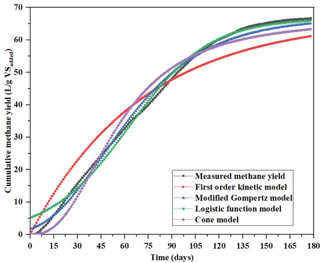
Fig. 7. Experimental data and model simulation/prediction of cumulative methane yield of daily feeding mode.
