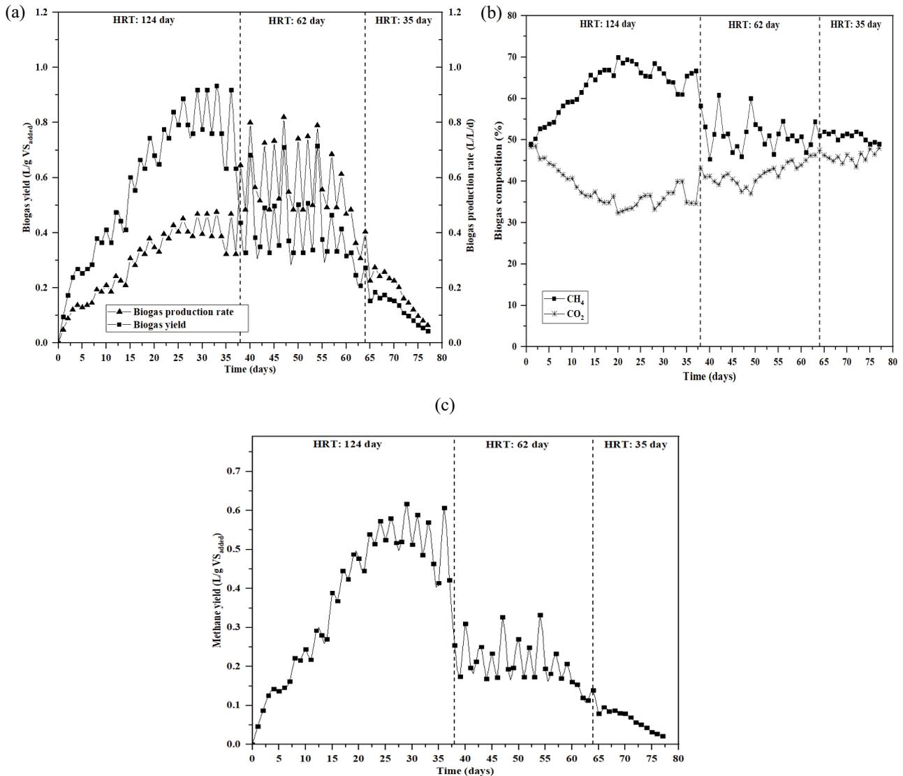
Fig. 2. (a) Biogas yield and biogas production rate, (b) biogas composition, and (c) methane yield in feeding mode 3-times-per-week during operation under declined HRTs.
