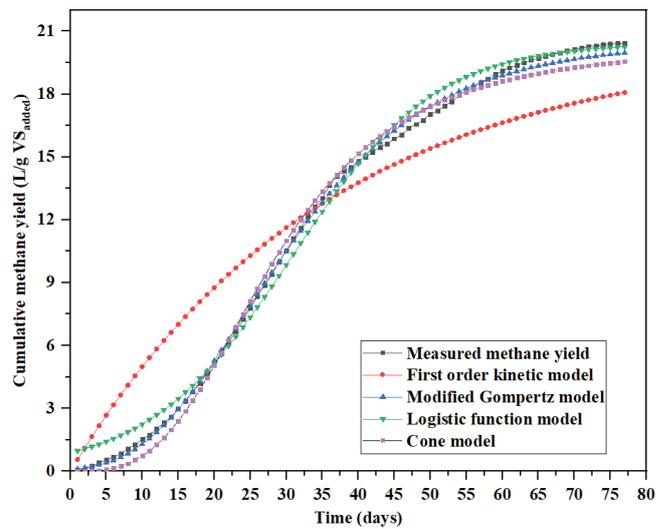
Fig. 8. Experimental data and model simulation/prediction of cumulative methane yield of 3-times-per-week feeding mode.
