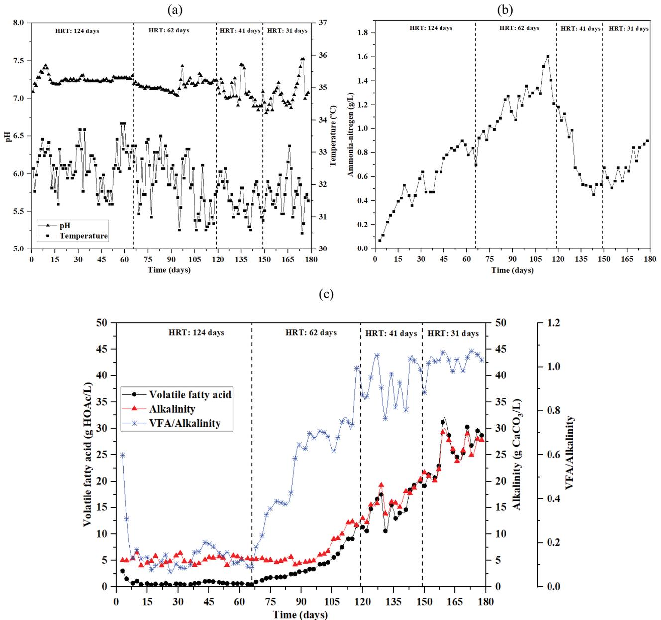
Fig. 3. (a) pH and temperature value, (b) ammonia-nitrogen concentration, and (c) volatile fatty acid and total alkalinity concentration in daily feeding mode during operation under declined HRTs.
