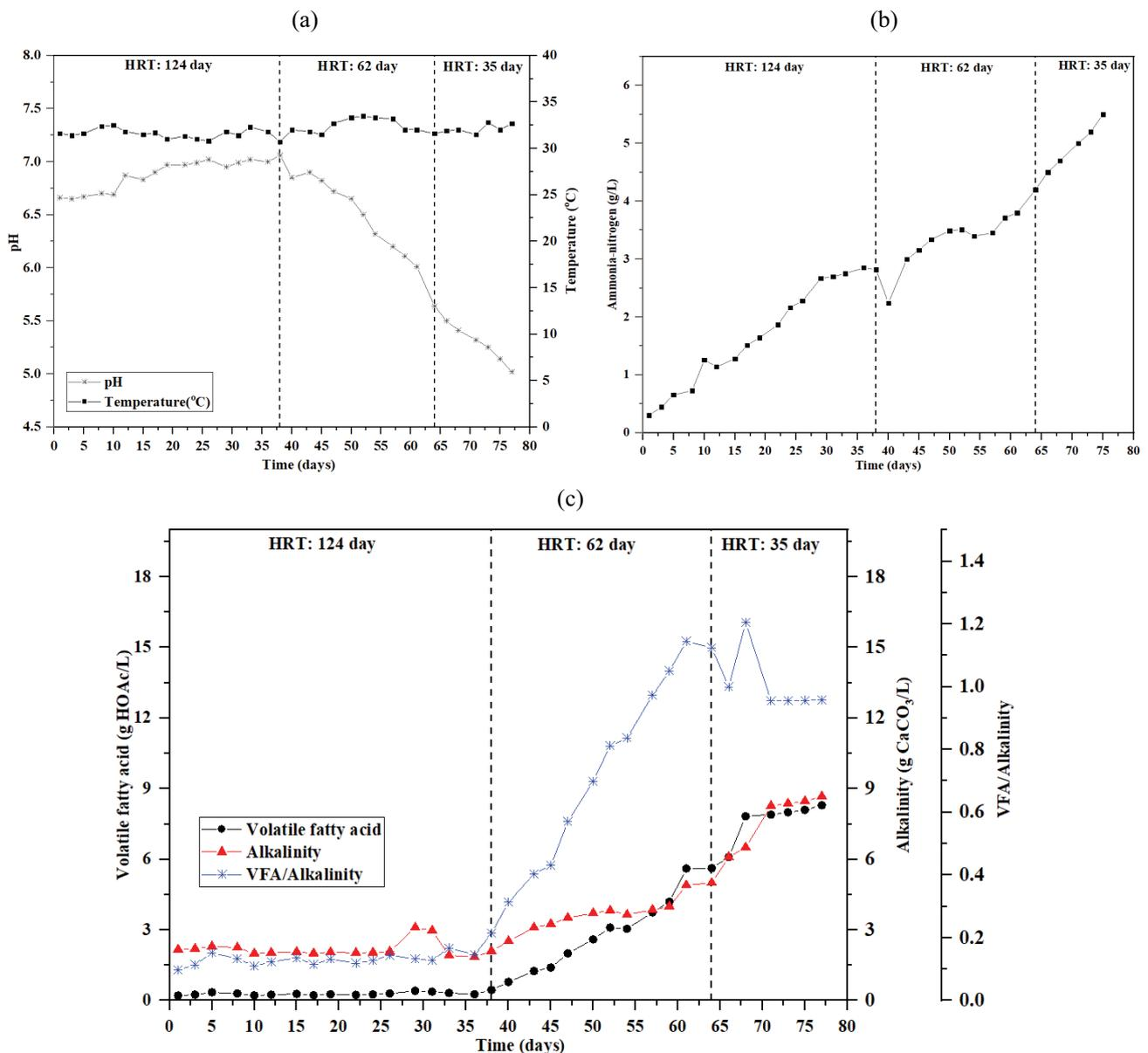
Fig. 4. (a) pH and temperature value, (b) ammonia–nitrogen concentration, and (c) volatile fatty acid and total alkalinity concentration; in feeding mode 3-times-per-week during operation under declined HRTs.
