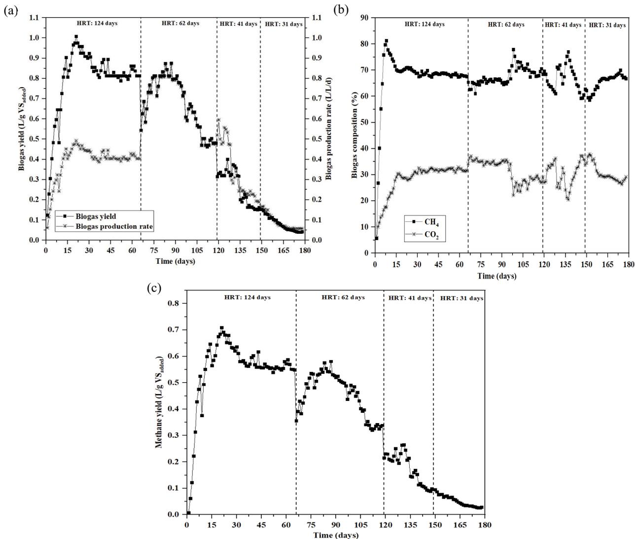
Fig. 1. (a) Biogas yield and biogas production rate, (b) biogas composition, and (c) methane yield in daily feeding mode during operation under declined HRTs.
