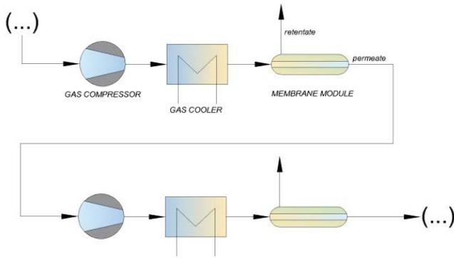
Fig. 2. Scheme of connections within the membrane separator, serial membrane connection (based on the study by Remiorz et al. [24]).
