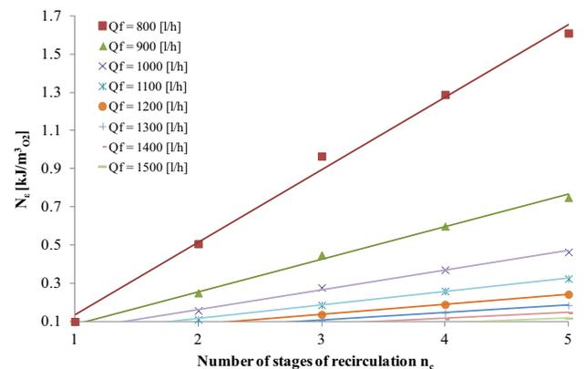
Fig. 9. Energy efficiency of the separation in the separator including retentate recirculation, as a function of feed flow and number of retentate recirculation cycles.
