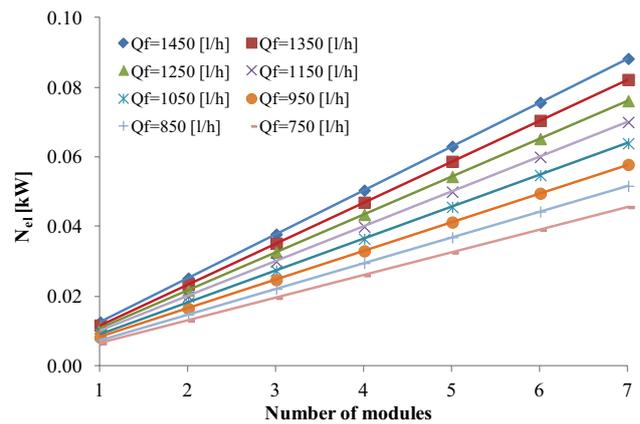
Fig. 5. Power demand of the separator, including serial connection of individual membranes, as a function of feed flow and number of modules in series.
