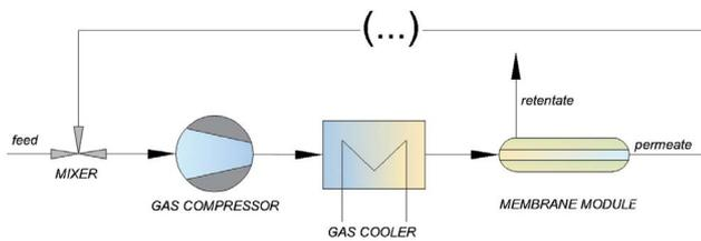
Fig. 4. Scheme of connections within the membrane separator, permeate recirculation (based on the study by Remiorz et al. [24]).
