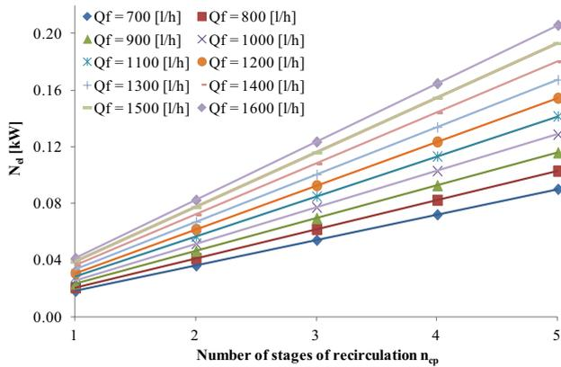
Fig. 10. Power demand of the separator including permeate recirculation, as a function of feed flow and number of permeate recirculation cycles.
