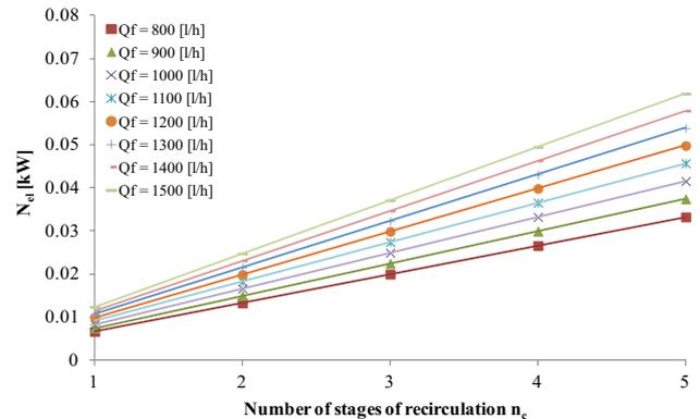
Fig. 8. Power demand of the separator including retentate recirculation, as a function of feed flow and number of retentate recirculation cycles.
