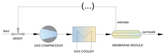
Fig. 3. Scheme of connections within the membrane separator, retentate recirculation (based on the study by Remiorz et al. [24]).
