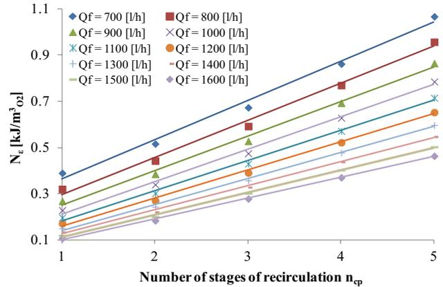
Fig. 11. Energy efficiency of the separation in the separator including permeate recirculation, as a function of feed flow and number of permeate recirculation cycles.
