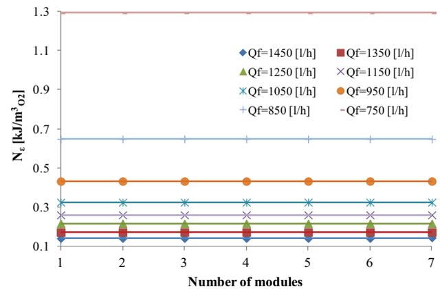
Fig. 6. Energy efficiency of the separation in the separator including serial connection of individual membranes, as a function of feed flow and number of modules in series.
