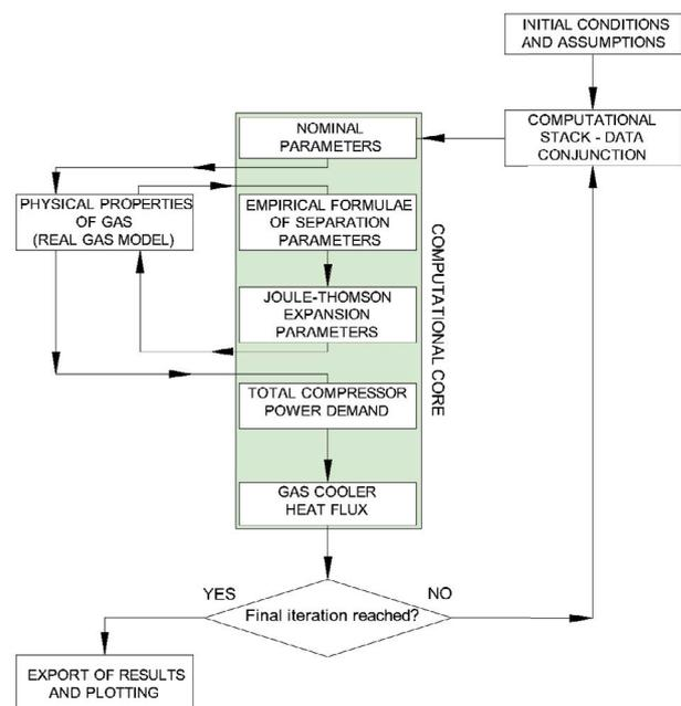
Fig. 1. Scheme of the computations performed within the applied model (based on the study by Remiorz et al. [24]).
