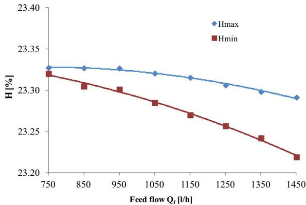
Fig. 7. Useful energy ratio of the separator including serial connection of individual membranes, as a function of feed flow and number of modules in series.
