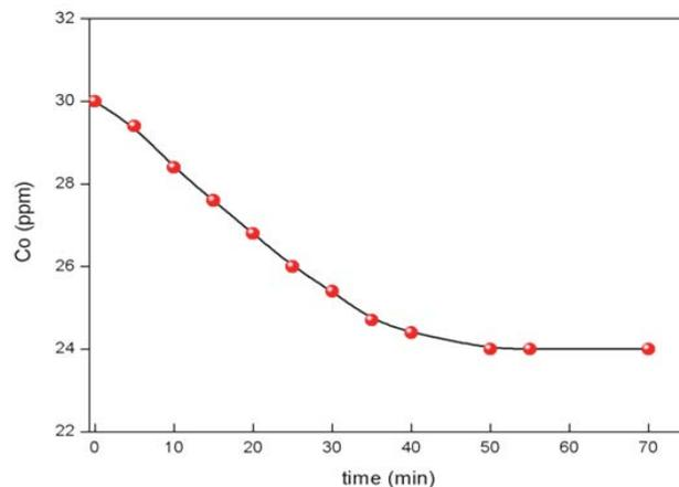
Fig. 3. Determination of the Methyl orange adsorption equilibrium time.
