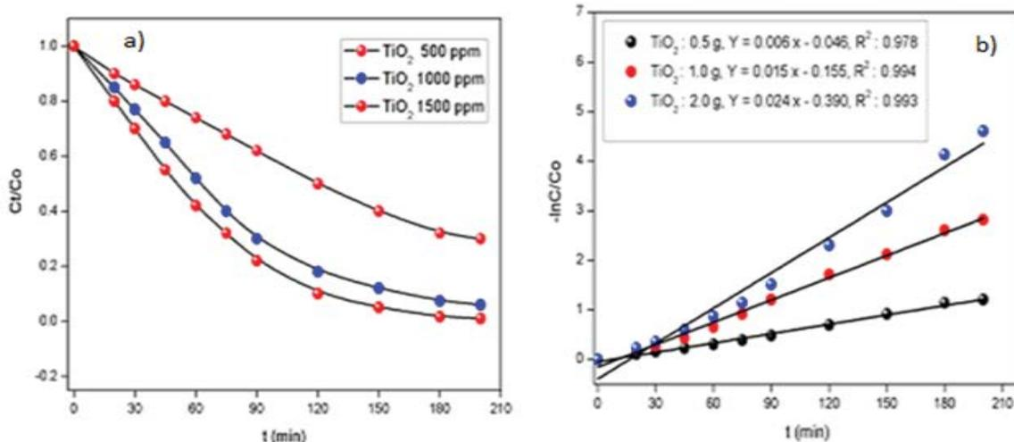
Fig. 5. Methyl orange degradation kinetics for different TiO<sub>2</sub> concentrations.
