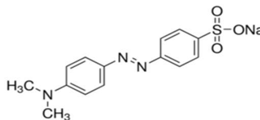
Fig. 1. Structure of Methyl Orange.
