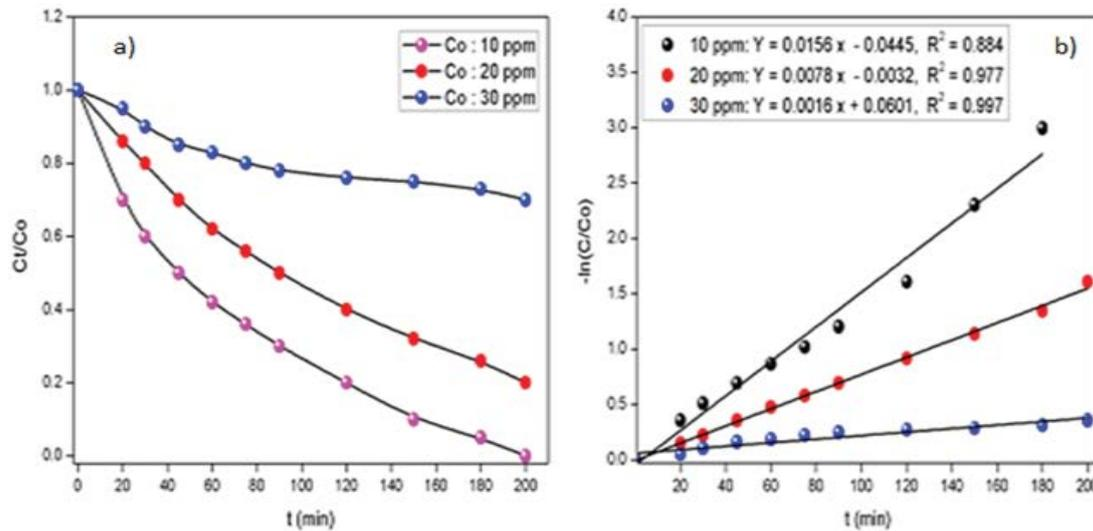
Fig. 4. (a) Methyl orange kinetics of degradation at different initial concentrations in the presence of  $\text{TiO}_2$  (1 g/L). (b) Modeling of the degradation kinetics of methyl orange according to the Langmuir–Hinshelwood model.
