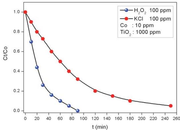
Fig. 7. Influence of  $\text{H}_2\text{O}_2$  and NaCl on the degradation kinetics of methyl orange in the presence of  $\text{TiO}_2$  (1 g/L).
