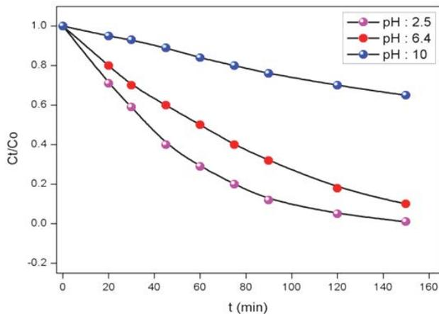
Fig. 6. Influence of pH on the degradation kinetics of methyl orange in presence of  $\text{TiO}_2$  (1 g/L).
