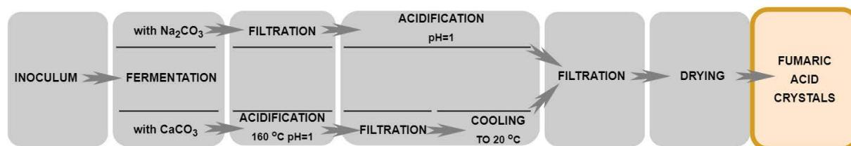
Fig. 8. Pathways of recovery of FA from fermentation broth using classical separation method (based on Martin-Dominguez et al. [72]).
