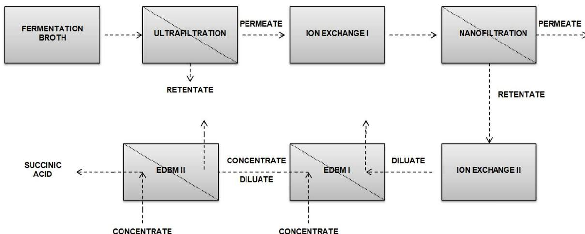
Fig. 6. General scheme of integrated membrane system used in the recovery of SA from fermentation broth (ultrafiltration – ion exchange (I) – nanofiltration – ion exchange (II) –EDBM I and EDBM II) based on Antczak et al. [15].
