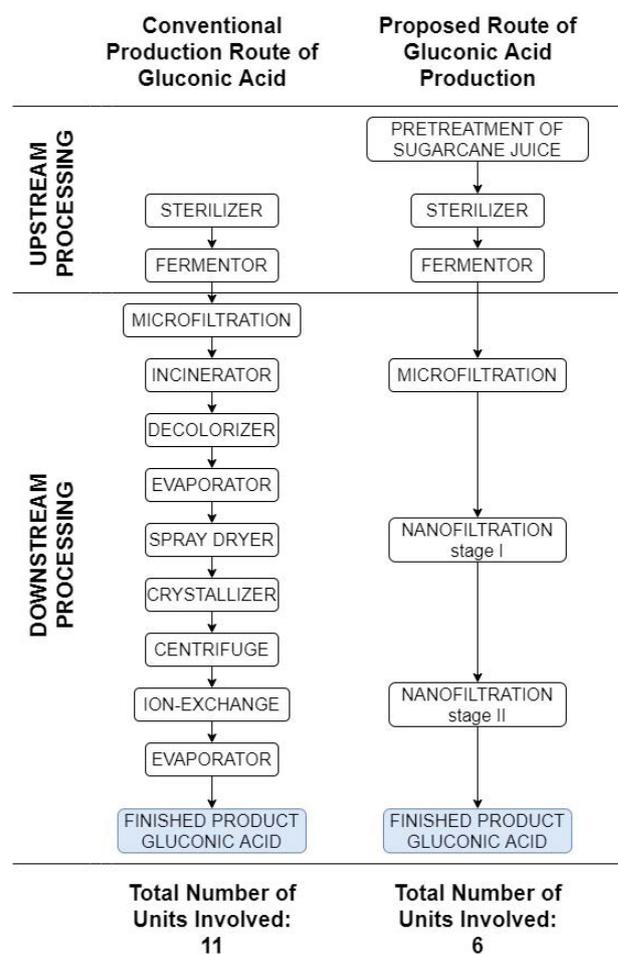
Fig. 11. Comparison of traditional (left) and membrane based (right) separation of GA from fermentation broth on the basis of Pal et al. [31].
