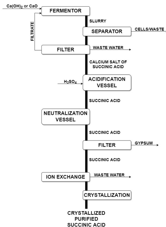
Fig. 4. Pathway of recovery of SA from fermentation broth using classical separation methods [51].
