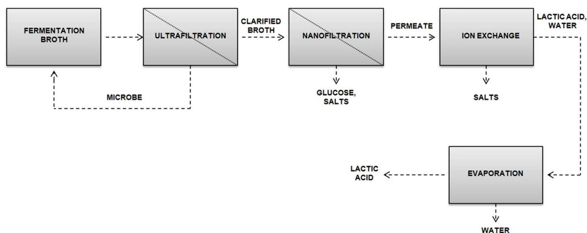
Fig. 2. General scheme of integrated membrane system used in the recovery of LA from fermentation broth (ultrafiltration – nanofiltration – ion exchange – evaporation) based on Lee et al. [19].
