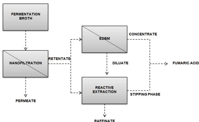
Fig. 9. General scheme of integrated membrane system used in the recovery of FA from fermentation broth (nanofiltration – EDBM – solvent extraction) based on Prochaska et al. [30].
