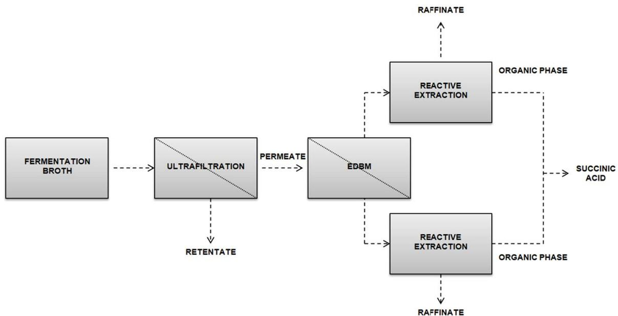
Fig. 5. General scheme of an integrated membrane system used in the recovery of SA from fermentation broth (ultrafiltration – EDBM – solvent extraction) based on Prochaska et al. [28].
