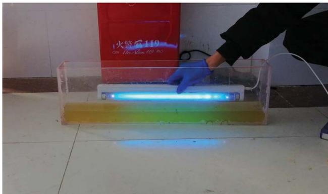
Fig. 1. Physical picture of the process of ultraviolet radiation on sewage treatment.
