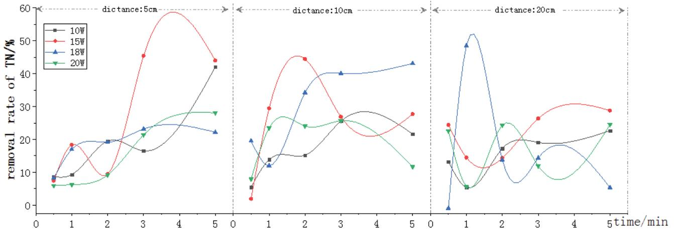
Fig. 3. Effect of UV radiation on TN removal.
