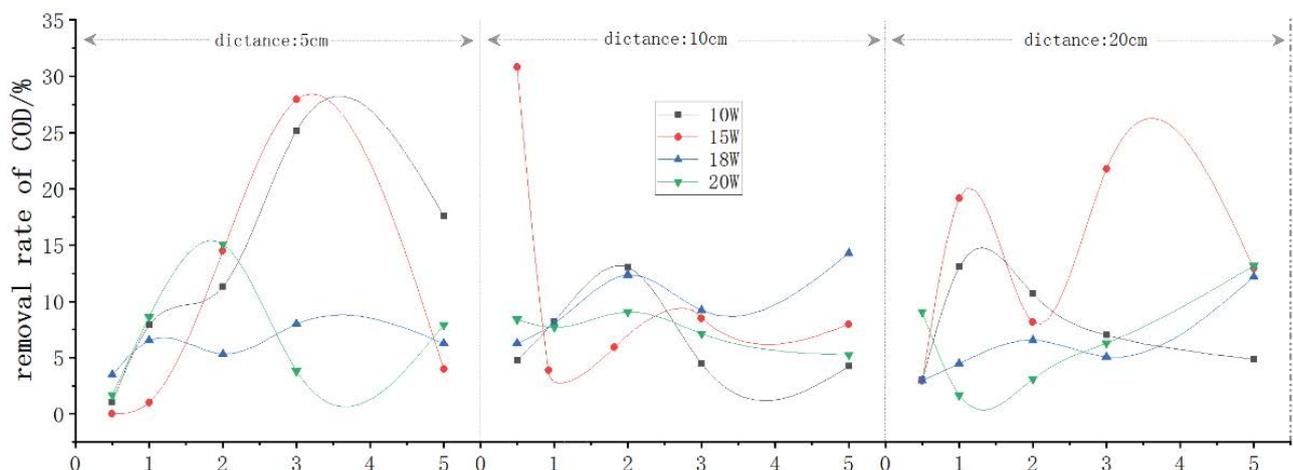
Fig. 2. Effect of UV radiation on COD removal.
