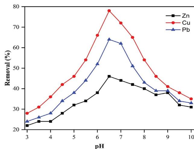
Fig. 2. Relationship between pH and ions removal.
