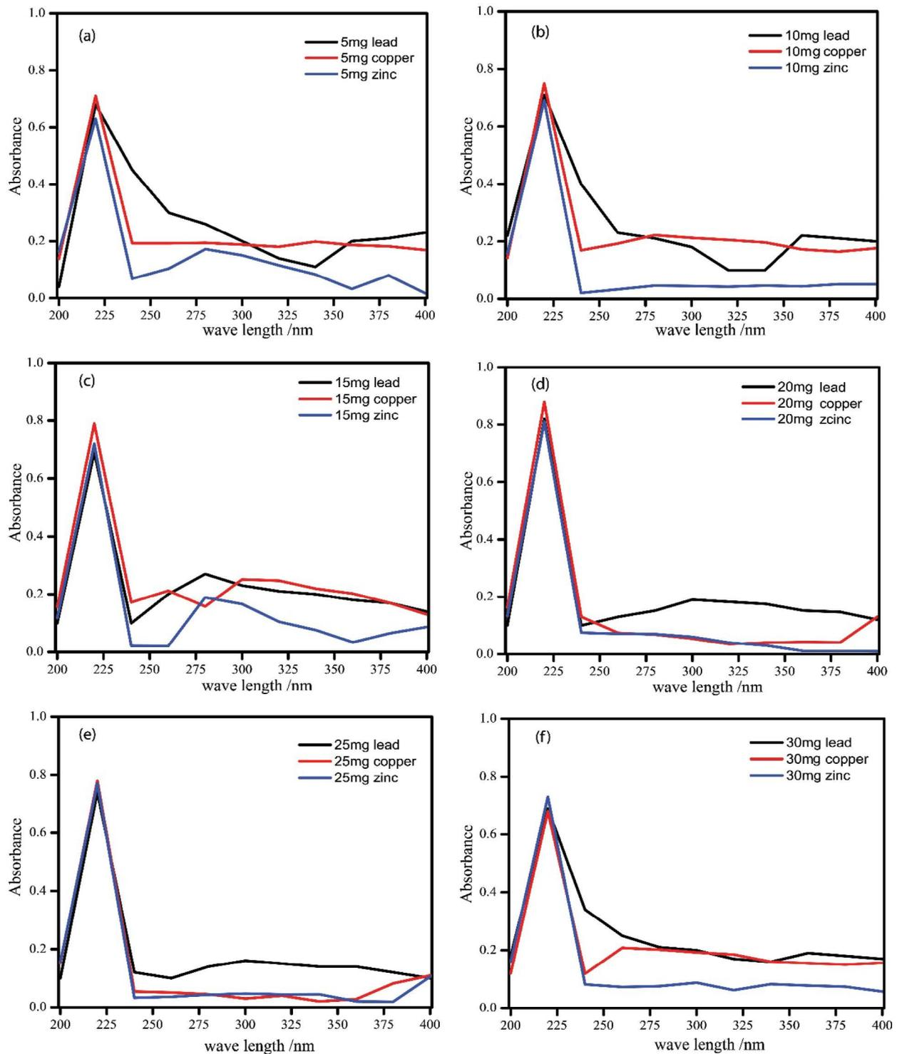
Fig. 3. UV-visible absorbance spectra of an aqueous solution of lead, copper, and zinc.
