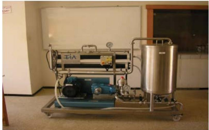
Fig. 1. Schematic diagram and picture of the nanofiltration/reverse osmosis pilot plant. T: tank; P: feed pump; V: pressure regulation valves; M: nanofiltration module; Pe: permeate recirculation; R: retentate recirculation; H: heat exchanger; 1: pressure sensor; 2: temperature sensor.
