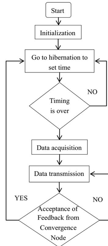
Fig. 2. Work flow of sensor node.
