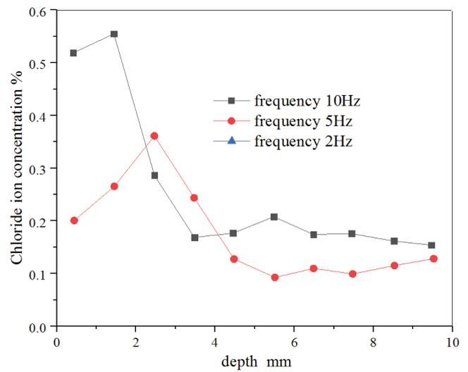
Fig. 4. Chloride corrosion of concrete under different loading frequencies at 0.5 load level.
