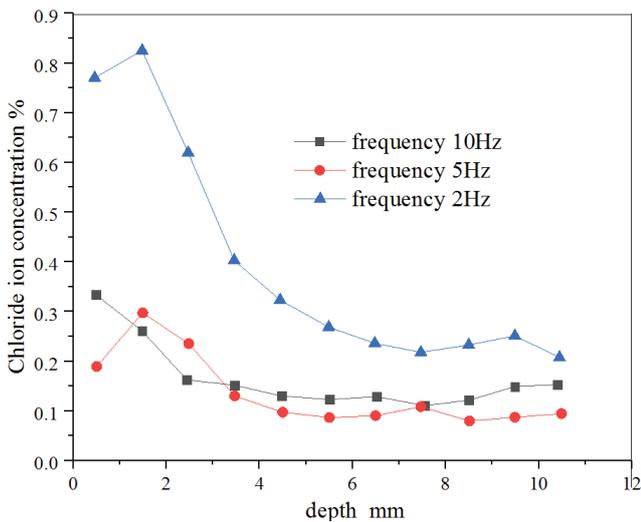
Fig. 3. Chloride corrosion of concrete under different loading frequencies at 0.3 load level.
