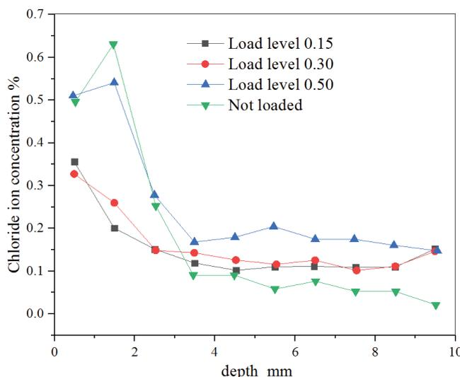
Fig. 1. Chloride ion erosion law of concrete structure under different load levels.
