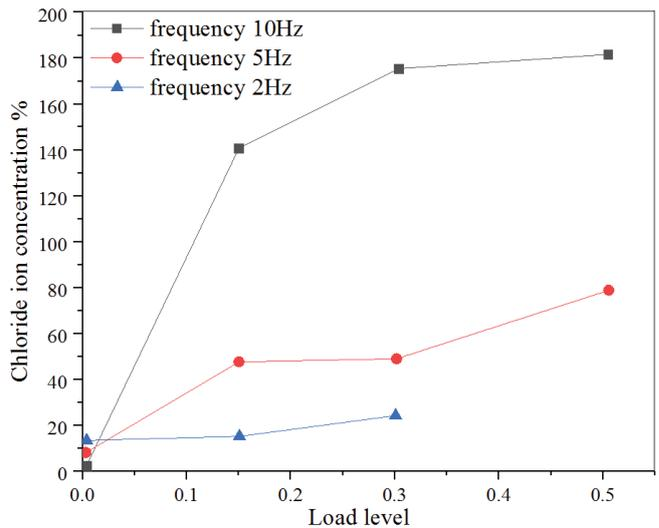
Fig. 5. Influence of horizontal loading frequency on the chloride diffusion coefficient of concrete at different load levels.
