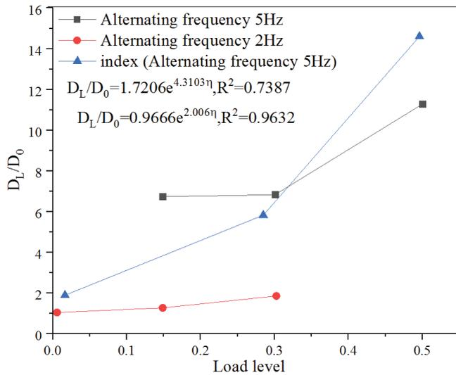
Fig. 6. Relation curve between the chloride diffusion coefficient of concrete and load level under the alternate frequency of 2 and 5 Hz.
