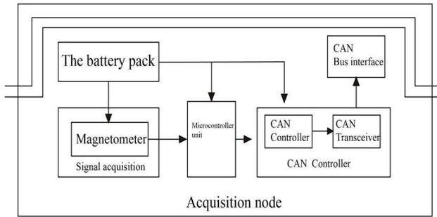
Fig. 1. Structure diagram of acquisition node.
