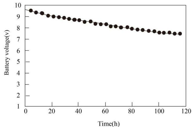
Fig. 6. Battery voltage consumption curve.
