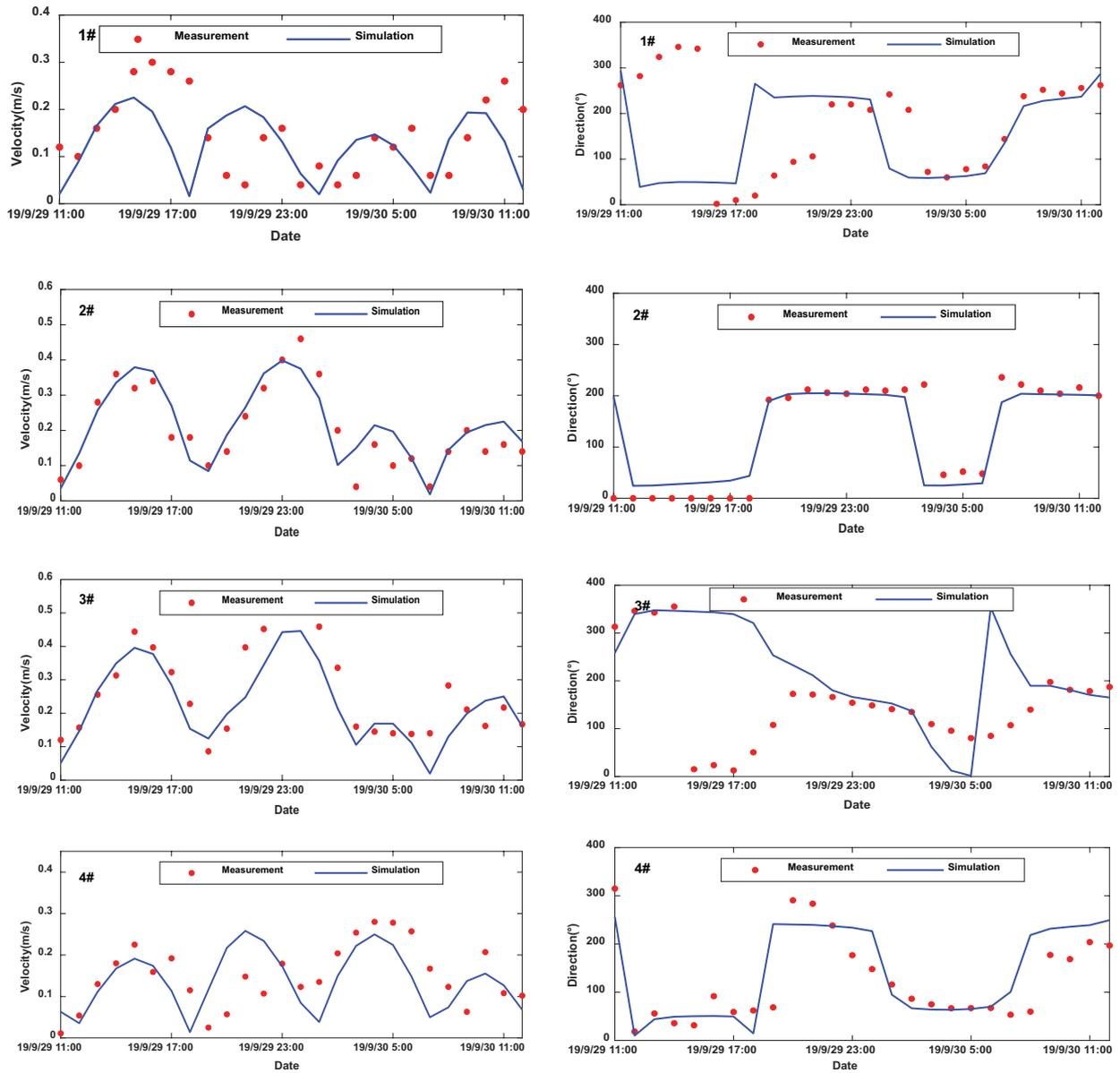
Fig. 4. Surface current verification curves in each stations.
