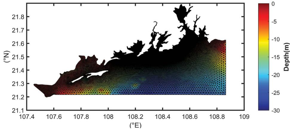
Fig. 1. Triangular system in modeled area and the distribution of depth.
