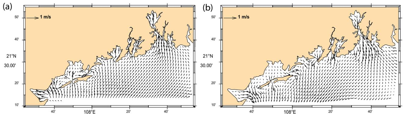
Fig. 5. Flow field of high (a) and low (b) tide during spring period.
